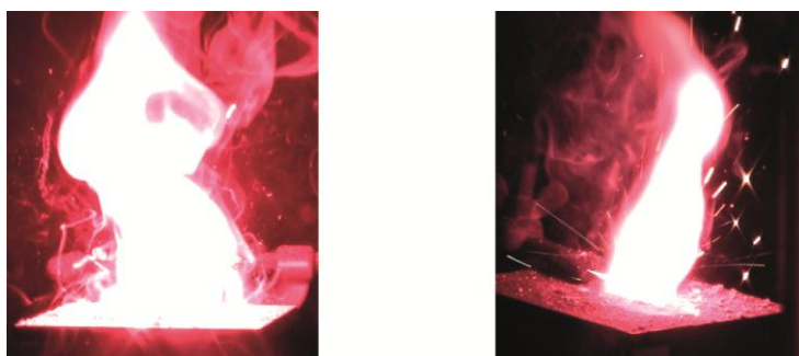
Figure I.4: Comparison of red flares containing harmful strontium and chlorinated materials (left) and environmentally benign composition featuring lithium and halogen-free substitutes (right).
