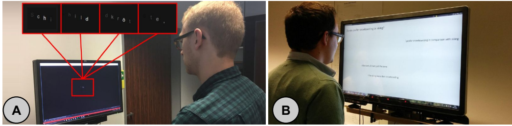
Figure 4.2: In our project TextPursuits, we implemented and evaluated two systems: (A) Read2Calibrate allows users to implicitly calibrate the eye tracker while reading text on public displays, and (B) EyeVote allows users to vote on public displays by picking one of several text-based options by following them with their eyes. Through two user studies, we identified several factors that influence the accuracy and user perception, as well as a trade-off between accuracy and perceived user experience.
