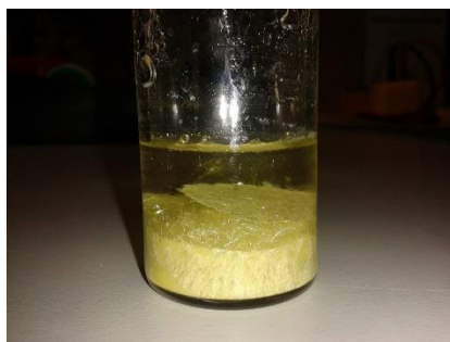
Figure 3.4 Photograph of synthesized crystals of (CH 3 NH 3 ) 4 PbI 6 · 2 H 2 O in the mother liquor.
