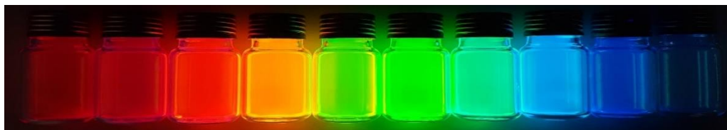
Figure 1.10 Photograph of cesium lead halide perovskite nanocrystal dispersions with varying halide compositions, yielding a broad range of fluorescence colors under UV-light illumination.
