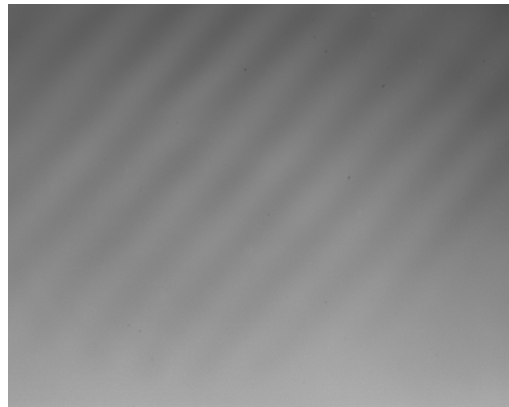
(d) WLI image of 35 nm target. The contrast in focal position is superior compared to the bright field image, which makes it easy to position this target in focal position.
