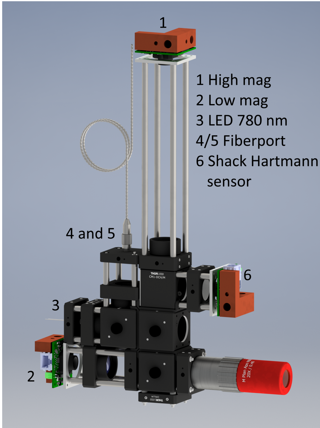
Figure 4.26: 3D model of the microscope for LION at CALA.
