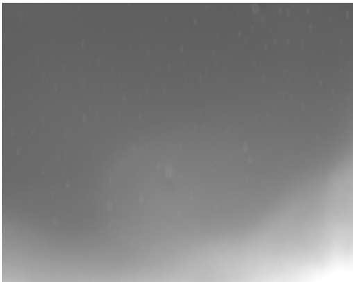
(c) Bright field image of 35 nm formvar target. The contrast is very low, which makes it difficult to position the target in focus.
