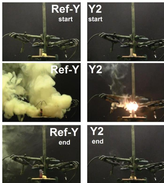
Figure 3: Burning of Ref-Y and Y2 with a pellet size of 3 g.
