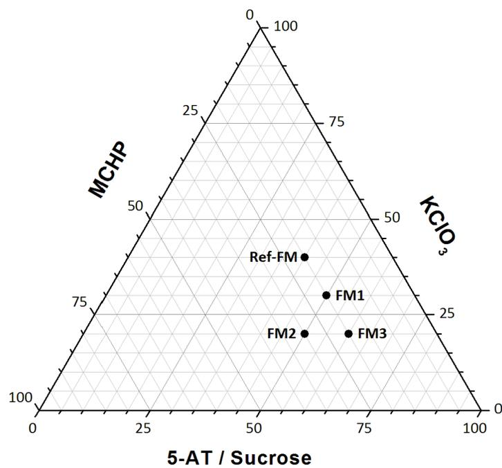
**Figure 2:** Developed fuel mixes. **FM1** = 5-AT (50 wt%),  $\text{KClO}_3$  (30 wt%), MCHP (20 wt%); **FM2** = 5-AT (50 wt%),  $\text{KClO}_3$  (20 wt%), MCHP (30 wt%); **FM3** = 5-AT (60 wt%),  $\text{KClO}_3$  (20 wt%), MCHP (20 wt%); **Ref-FM** = sucrose (40 wt%),  $\text{KClO}_3$  (40 wt%), MCHP (20 wt%). See Table 2 and Table 3 for a complete listing of formulation ingredients, weight percentages and the ESI for brief explanation of the triangle diagram.
