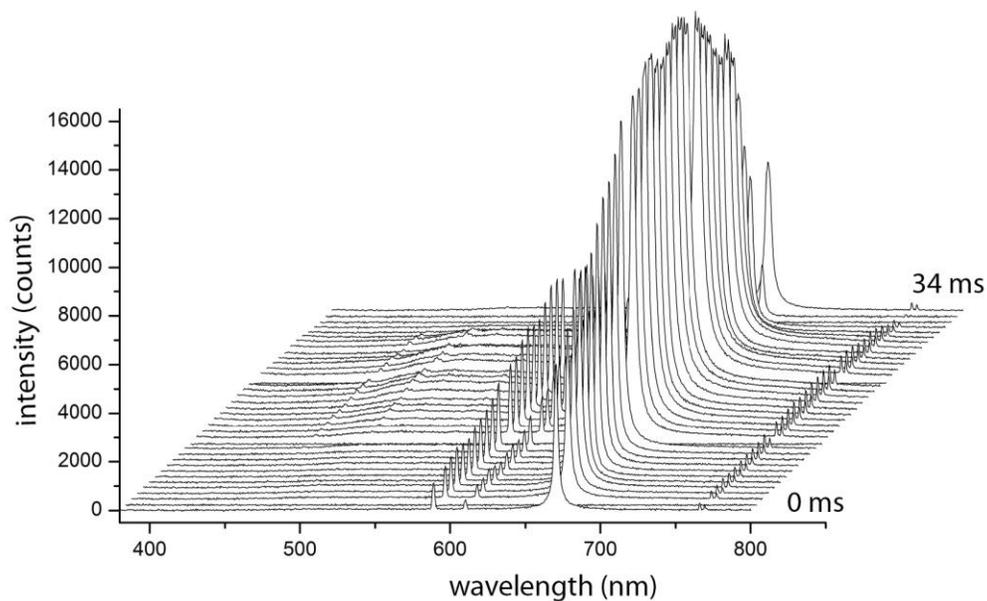
**Figure 5.** Time dependent high-speed measurement of formulation 6 (1 ms/scan).
