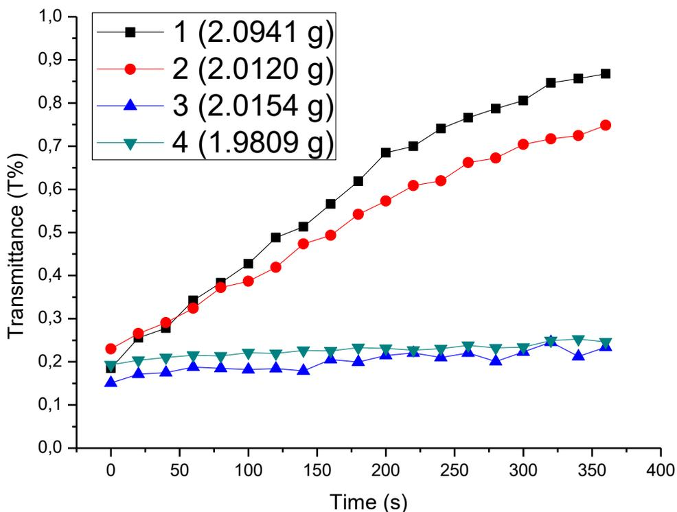
**Figure 2.** Transmittance (555 nm) over time for a representative pellet of each composition
