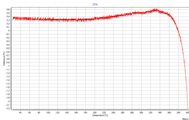
Figure 12. DTA (5°C/min) of terephthalic acid
