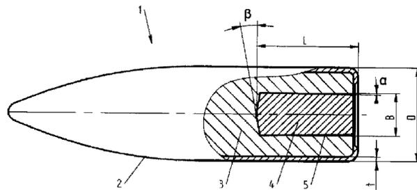
**Figure 6.** Scheme of tracer ammunition for small- and medium-calibre weapons. (1 = jacketed tracer projectile; 2 = bullet; 3 = metal core; 4 = tracer device; 5 = cavity for the tracer ammunition which is usually pressed in an additional sleeve).<sup>[26]</sup>
