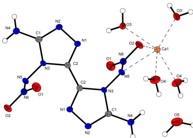
**Figure 7.** Molecular unit of **7** showing the atom-labeling scheme. Ellipsoids represent the 50% probability level. Symmetry codes: (*i* = 0.5+*x*, 0.5+*y*, *z*). Selected bond length (Å): Ca1-O2 2.4801(14), Ca1-O3 2.3797(14), Ca1-O4 2.3614(1), Ca1-N5 2.5785(1).
