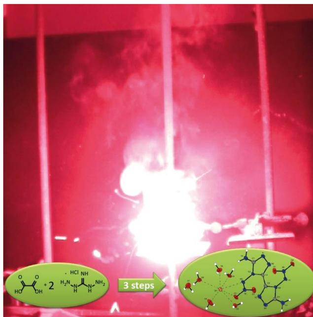
**Figure 11.** Red pyrotechnical formulation based on  $SrANAT \cdot 6H_2O$ .
