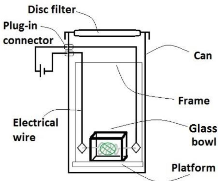
**Figure 4.** Scheme aerosol collecting setup.
