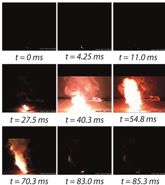
**Figure S9.** High speed video recording of formulation C (4000 frames per seconds).
