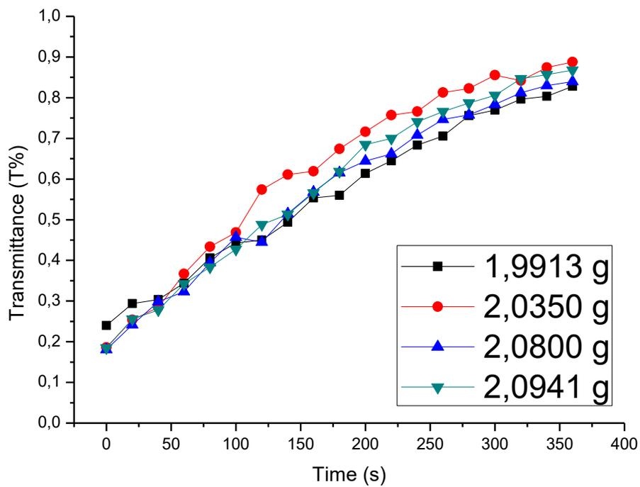
Figure 1. Transmittance (555 nm) over time of formulation 1
