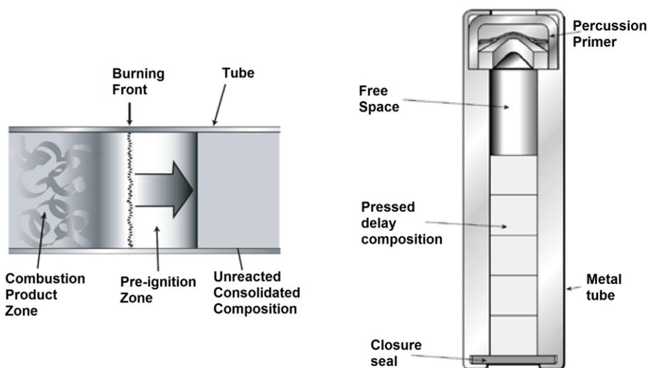
**Figure 5.** Schematic burning of the ignited delay composition within the tube (left) and delay element scheme (right).<sup>[21]</sup>
