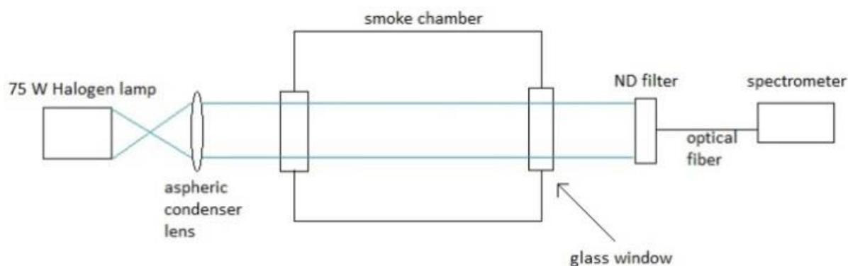
**Figure 3.** Setup for optical measurement designed by Poret and suggested by Shaw <sup>[24]</sup>.
