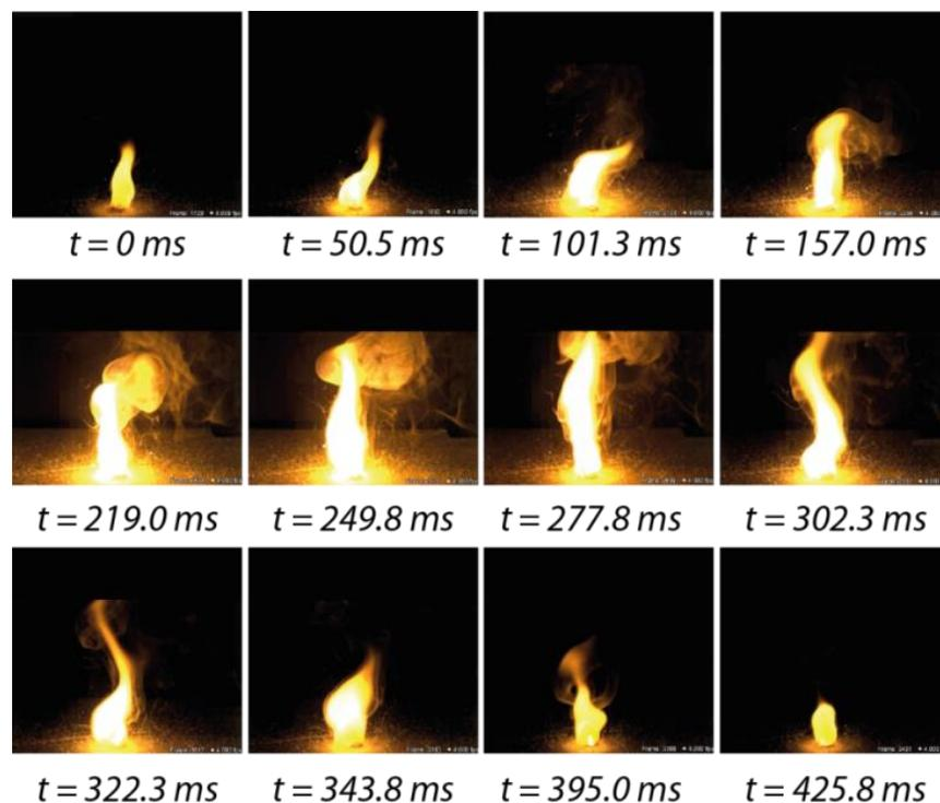
**Figure 3.** Time-resolved images of the burning of a strobe pellet (composition **4** in Table 2).
