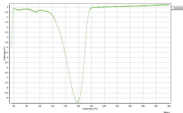
**Figure 16. DTA (5°C/min) of NaHCO<sub>3</sub>, measurement started at elevated temperatures (60 °C), no decomposition before 60 °C**
