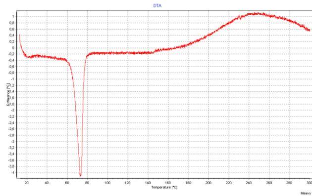
Figure 14. DTA (5°C/min) of stearic acid
