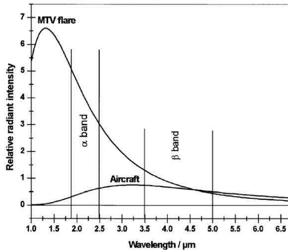
**Figure 7.** Comparison of relative magnitude of both MTV and target radiant intensity.<sup>[34]</sup>
