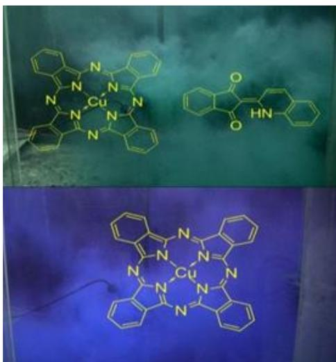
**Figure 8.** Copper(II) phthalocyanine (bottom) and Solvent Yellow 33 (top right) applied in new green and blue smoke formulations.
