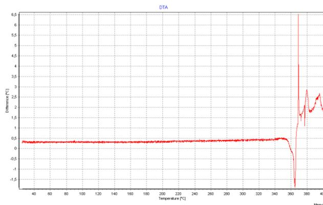
**Figure 9. DTA (5°C/min) of KClO<sub>3</sub>**
