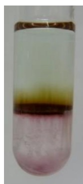
Figure 1.8: The “brown-ring test”. The tentative chromophore of the “brown ring”, [\text{Fe}(\text{H}_2\text{O})_5\text{NO}]^{2+} , is a well-known representative of \{\text{FeNO}\}^7(S=3/2) complexes. The picture is presented with kind permission from Prof. Dr. Peter Klüfers.
