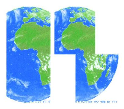
**Figure 3.1:** The HRV aboard MSG/SEVIRI covers only half of the earth in the E-W direction with  $11\ 136\times 5568$  pixels; however, the area of imaging can be selected [Schmetz et al., 2002].
