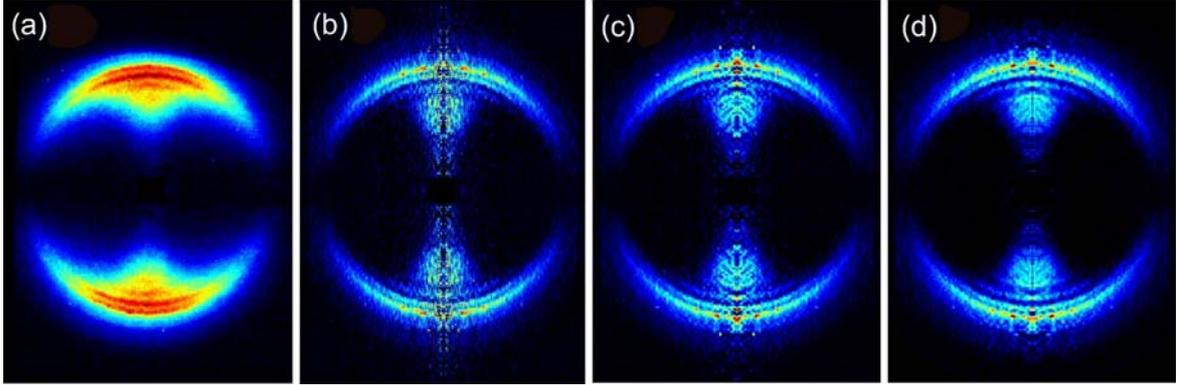
Figure 3.10: (a) Measured 2D projection of the velocity distribution of the fragments from photodissociation of  $D_2^+$  at an intensity of  $3.5 \times 10^{13} \text{ W/cm}^2$ . Cuts through the 3D velocity distribution reconstructed using: (b) Fourier-Hankel method (AbelWin package [96]); (c) BASEX method [97]; (d) iterative procedure of Vrakking [98].
