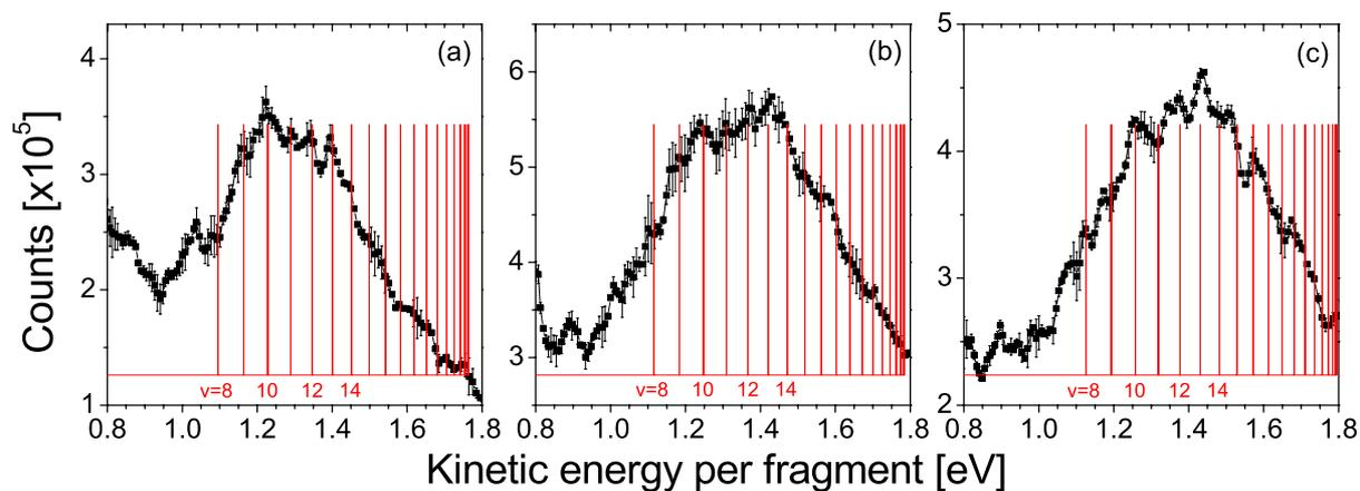
Figure 6.11: Comparison of the spectra of  $\text{D}_2^+$  from Fig. 6.9 with the one-photon vibrational “comb”. The peak intensities are (a)  $6.4 \times 10^{13}$ , (b)  $7.5 \times 10^{13}$  and (c)  $7.8 \times 10^{13}$   $\text{W}/\text{cm}^2$ . The “combs” were shifted by (a) 0.98 eV, (b) 1.0 eV and (c) 1.01 eV from its dissociation position, corresponding to ionization at critical distances of  $R_c \sim 13.5$ – $13.9$  a.u.
