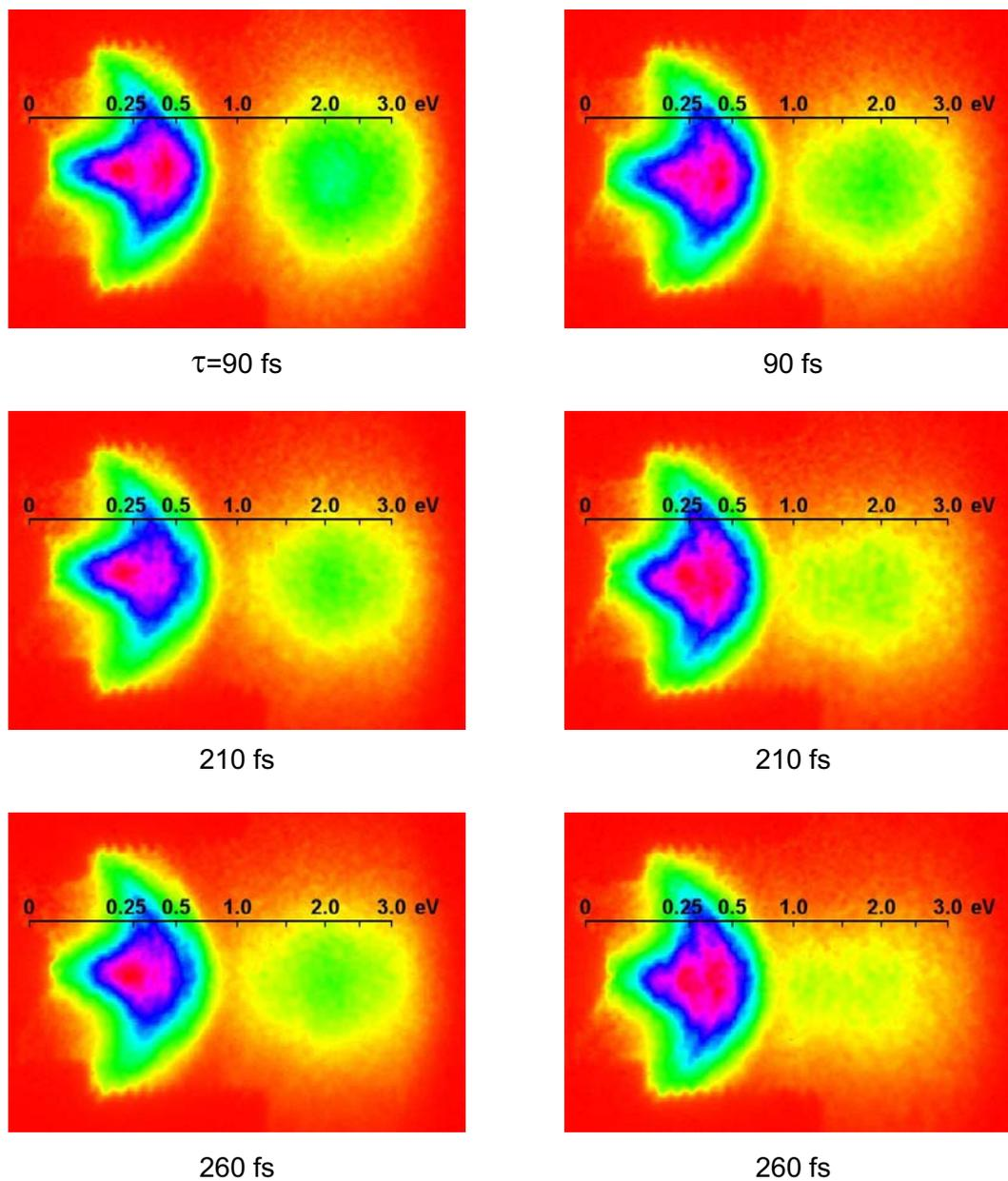
Figure 6.13: Projected 2D velocity distributions from photodissociation and Coulomb explosion of  $D_2^+$  (left) and  $H_2^+$  (right) for different pulse durations ( $\tau$ ). The pulse energy of 1.7 mJ was the same in all measurements. The peak intensities range from  $4 \times 10^{14}$  down to  $5 \times 10^{13}$  W/cm<sup>2</sup>.
