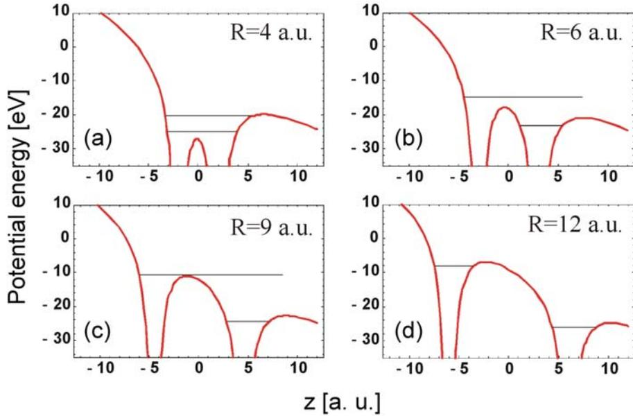
Figure 2.6: Potential energy of the electron in the combined field of two protons (located at  $-R/2$  and  $R/2$ ) and a static electric field [Eq. (2.20)]. The amplitude of the electric field is  $E_0 = 0.06$  a.u. ( $I \sim 1.2 \times 10^{14}$  W/cm<sup>2</sup>). The horizontal lines mark the energies of the two lowest electronic states of H<sub>2</sub><sup>+</sup> in the resulting potential.
