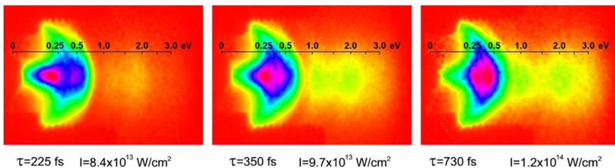
Figure 6.17: Projected 2D velocity distributions of the Coulomb explosion fragments of  $D_2^+$  at different pulse durations ( $\tau$ ) and similar peak intensities ( $I$ ).
