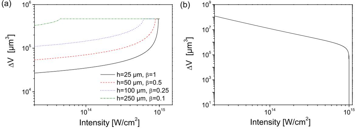
Figure 3.20: Volume of iso-intensity shells with  $\Delta I/I = 0.1$  as a function of intensities in the interaction region. (a) ion beam of width  $l = 300 \mu\text{m}$  and different widths  $h$  [Eq. (3.32)]; (b) no constraints on the interaction volume [Eq. (3.33)]. The laser peak intensity and beam width are  $I_0 = 1 \times 10^{15} \text{ W}/\text{cm}^2$  and  $w = 30 \mu\text{m}$ , respectively.
