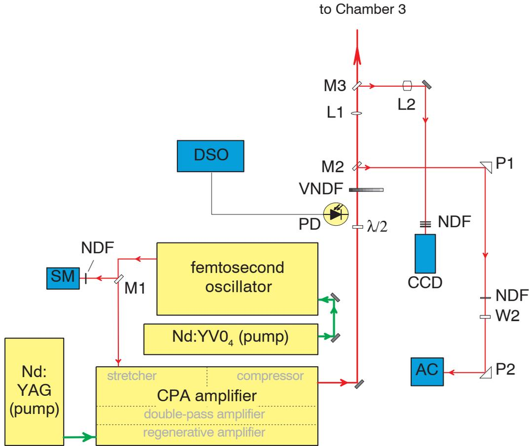
Figure 3.11: Layout of the femtosecond laser system. M, mirrors in flipper mounts; NDF, neutral density filter; SM, spectrometer;  $\lambda/2$ , half-wave plate; PD, photodiode; DSO, digital storage oscilloscope; VNDF, variable neutral density filter; L, lenses; P, prisms; W, window; AC, autocorrelator; CCD, CCD camera.
