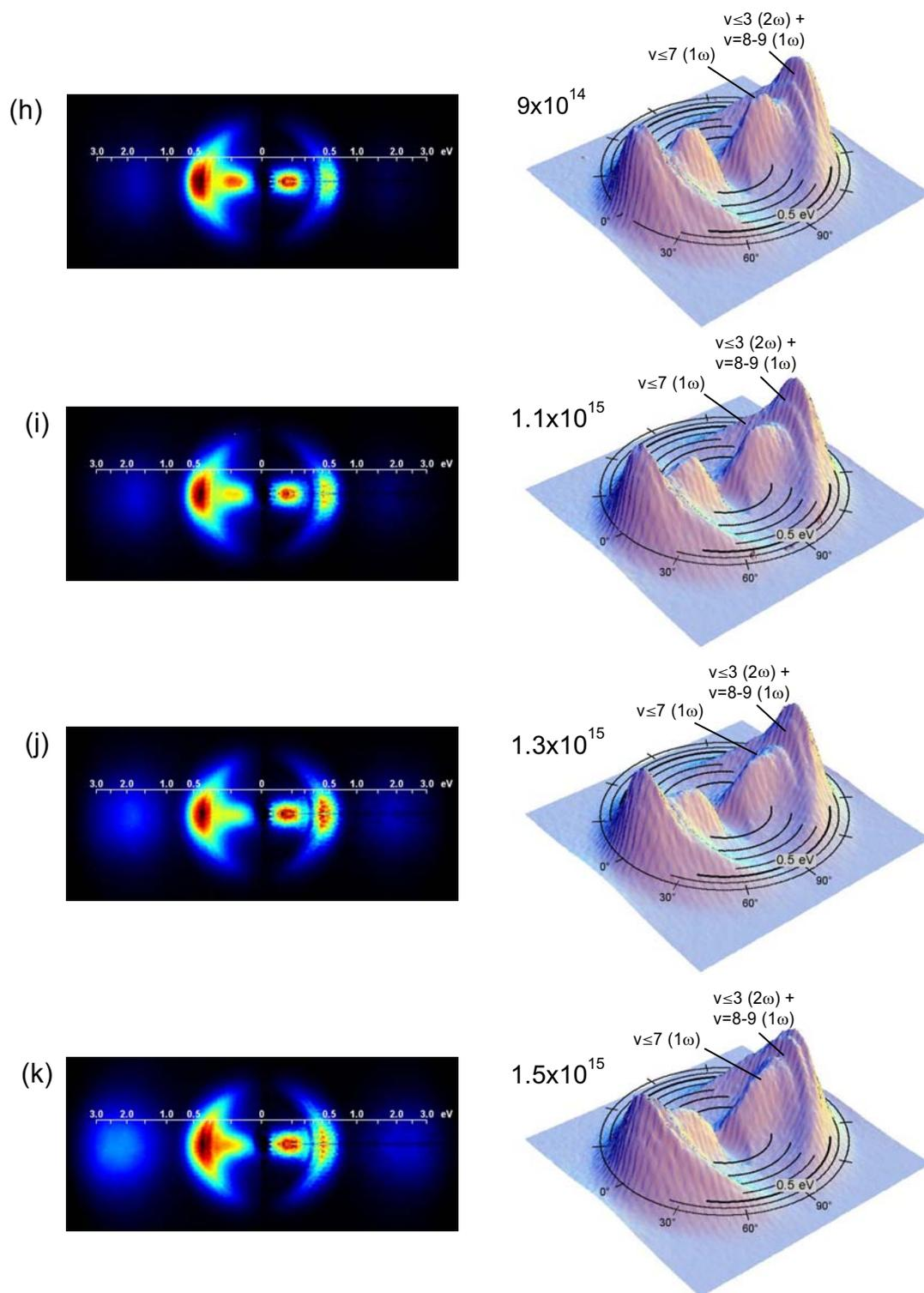
Figure 5.2 (continued): Velocity distributions of the fragments resulting from photodissociation and Coulomb explosion of  $\text{H}_2^+$  at different peak intensities.
