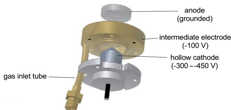
Figure 3.2: Drawing of the duoplasmatron ion source. Neutral gas introduced in the ion source through the inlet tube is ionized by electrons emitted from the hollow cathode. The produced plasma is confined by the electric field of the intermediate electrode and a nonuniform magnetic field of the intermediate electrode and a solenoid magnet. The electrodes are insulated by intermediate ceramic rings (not shown in the figure).
