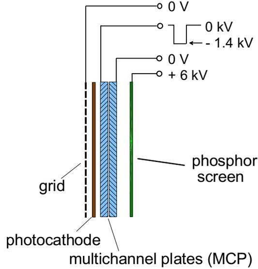
Figure 3.4: Schematic of the two-stage multichannel plate detector with the typical operating voltages.
