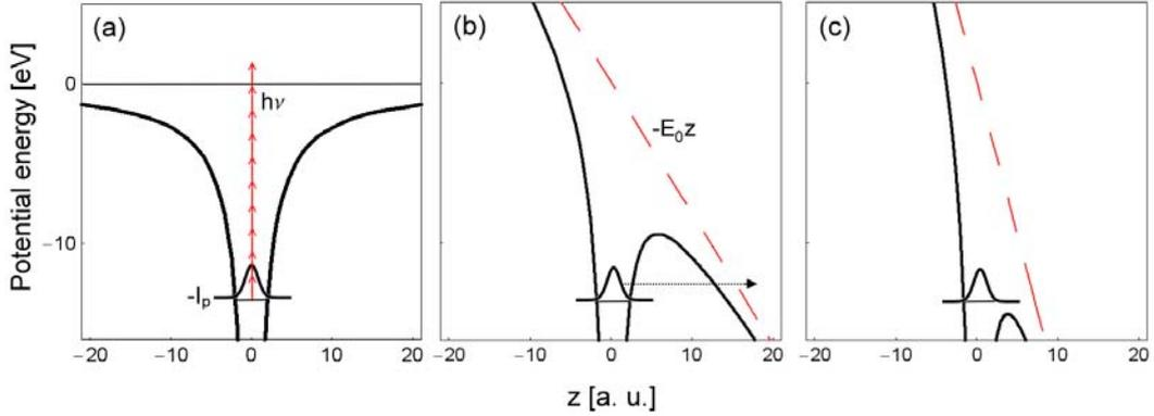
Figure 2.5: Schematic illustration of different mechanisms of atomic ionization: (a) multiphoton ionization, (b) tunnelling ionization and (c) over-the-barrier ionization.
