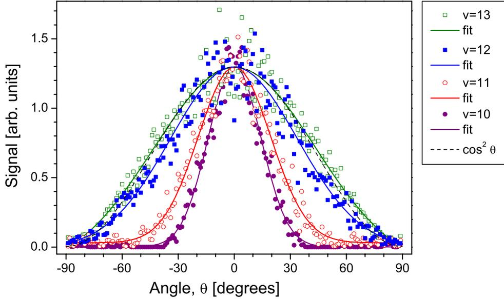
Figure 4.5: Angular distributions of the fragments from the vibrational levels  $v = 10$  to  $v = 13$ , as extracted from the inverted image in Fig. 4.2(a). Each angular distribution is averaged over five adjacent radii to minimize the noise. The solid curves show fits to Gaussian distributions of FWHMs given in Table 4.2, together with the corresponding alignment parameters  $\langle \cos^2 \theta \rangle$ . Here  $\theta$  is the angle between the molecular and the laser polarization axis.
