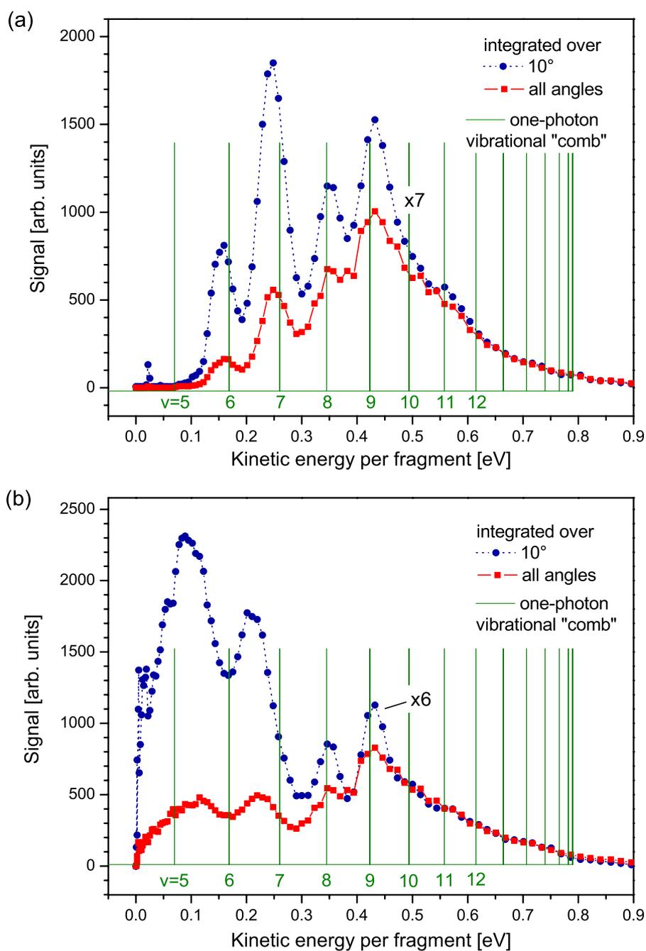
Figure 4.10: Fragment kinetic energy distributions from the inverted images in Fig. 4.9. The data were integrated over  $10^\circ$  and over all angles. The peak laser intensities and pulse durations are (a)  $3.5 \times 10^{13}$  W/cm<sup>2</sup>, 575 fs; (b)  $1.5 \times 10^{14}$  W/cm<sup>2</sup>, 135 fs.
