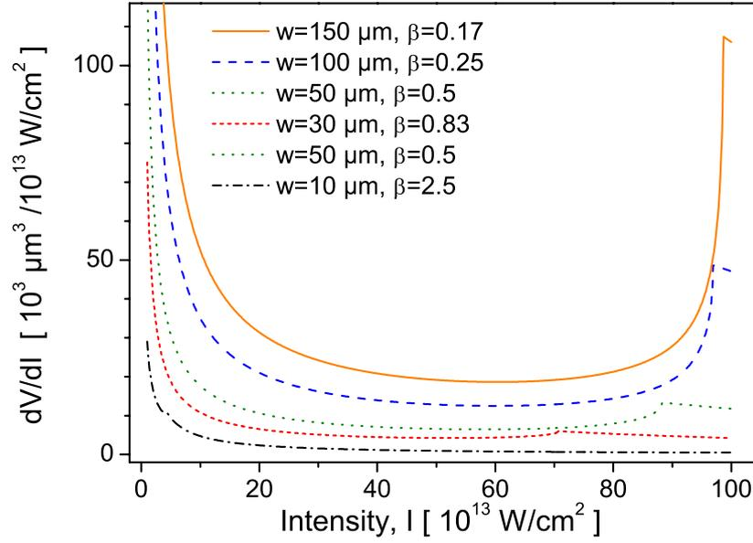
Figure 3.19: The gradient change of the volume of intensity shells,  $dV/dI$ , as a function of the intensity of the shells [Eq. (3.31)]. The calculations were made for the peak laser intensity  $I_0 = 1 \times 10^{15} \text{ W/cm}^2$ , and the ion beam dimensions of  $h = 25 \text{ } \mu\text{m}$  and  $l = 300 \text{ } \mu\text{m}$ . The curves are results of calculations for different laser beam widths, i.e., different parameters  $\beta = h/w$ .
