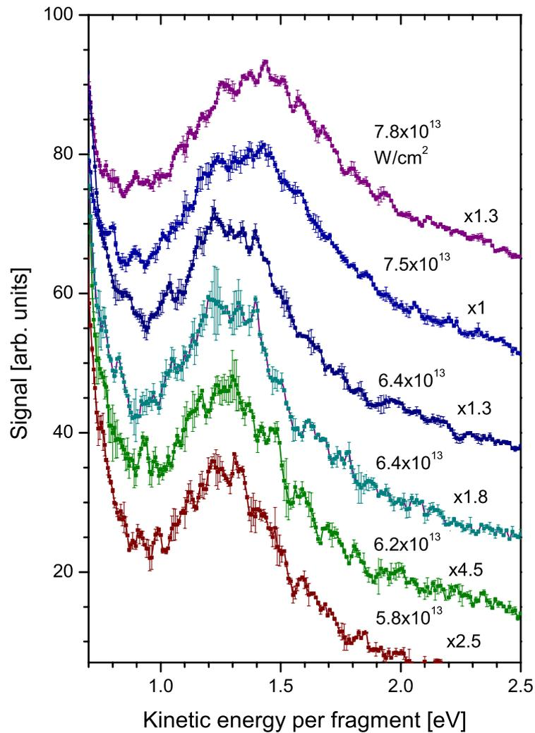
Figure 6.9: Kinetic energy spectra of deuterons in the Coulomb explosion channel of  $D_2^+$ . The spectra were obtained by integrating the projected 2D velocity distributions over  $2^\circ$  around the laser polarization axis. The pulse length was approximately 100 fs. The peak laser intensities and the scaling factors are given for each measurement.
