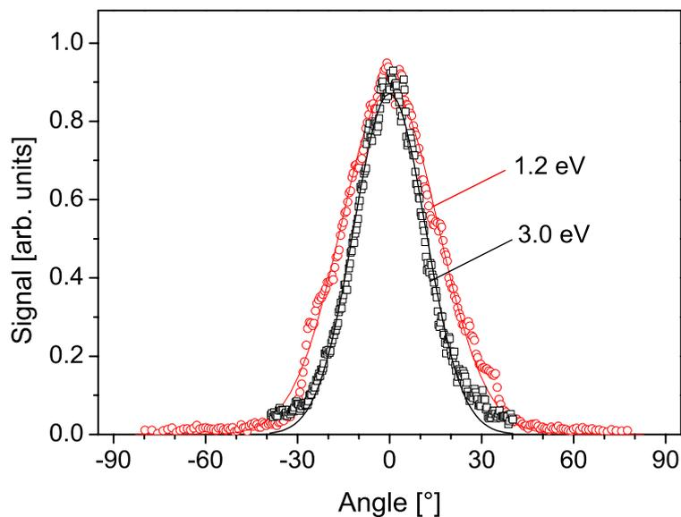
Figure 6.16: Angular distributions of the Coulomb explosion groups of  $D_2^+$  at kinetic energies of 1.2 and 3.0 eV. The data were extracted from the measurement with a pulse duration of 350 fs and a peak intensity of  $9.8 \times 10^{13} \text{ W/cm}^2$  (see Fig. 6.13). The solid lines are fits by Gaussian distributions with FWHMs of  $37^\circ$  at 1.2 eV and  $28^\circ$  at 3.0 eV.
