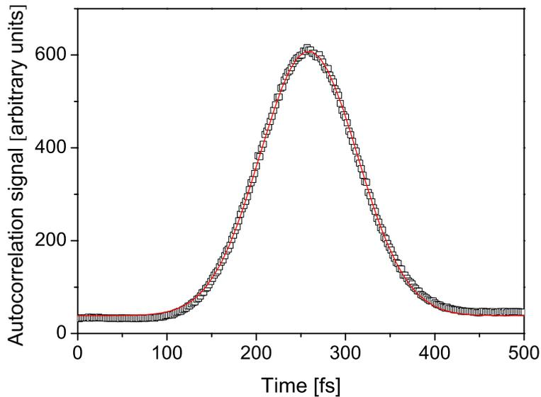
Figure 3.12: Autocorrelation function. The solid line is a fit to a Gaussian distribution corresponding to the pulse duration of  $\tau_p = 91$  fs.
