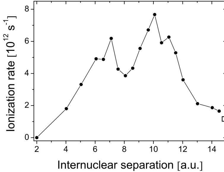
Figure 2.7: Ionization rate of  $\text{H}_2^+$  as a function of internuclear separation for a wavelength of 1064 nm and an intensity of  $1 \times 10^{14} \text{ W/cm}^2$ . The square on the right vertical axis marks the ionization rate of the hydrogen atom. The data were taken from [36].
