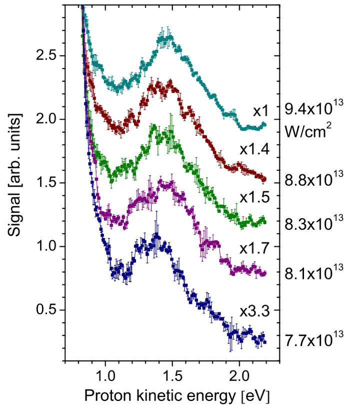
Figure 6.8: Kinetic energy spectra as in Fig. 6.6(a), but with the integration performed over angles in the range of  $2\text{--}4^\circ$  both above and below the symmetry axis.
