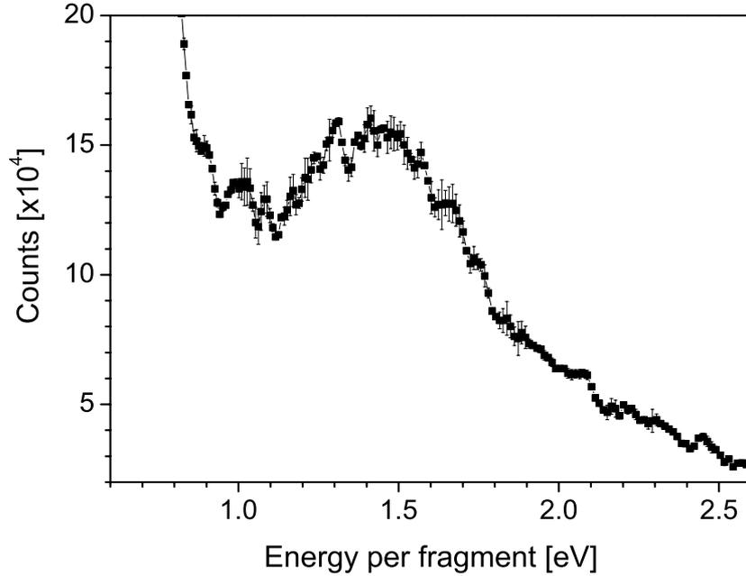
Figure 6.12: Coulomb explosion spectra of  $\text{H}_2^+$  with an elliptically polarized light of the ellipticity parameter  $\varepsilon = 0.29$ . The peak intensity was  $9.4 \times 10^{13} \text{ W/cm}^2$  and the pulse duration was 101 fs.
