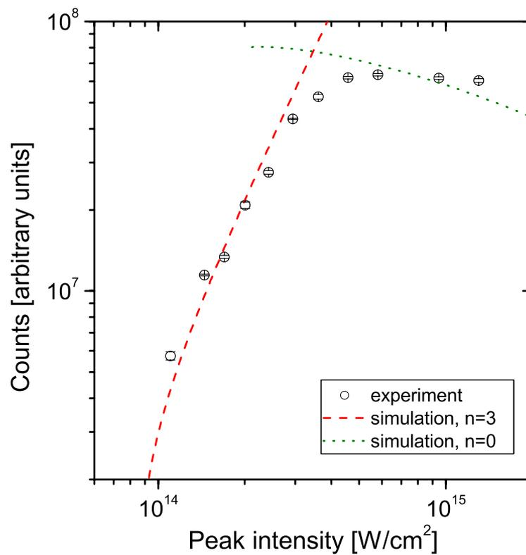
Figure 6.18: Yield of the Coulomb explosion fragments of  $H_2^+$  as a function of the peak laser intensity. The error bars were calculated from the standard deviation of data recorded in 2–3 measurements, each with  $\sim 4 \times 10^5$  laser shots. The pulse duration was 95 fs. The curves are results of the simulation of a  $I^n$  dependency, as described in Section 5.3.
