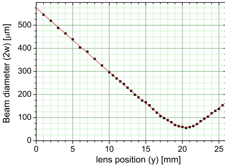
Figure 3.14: The variation of the laser beam diameter in the interaction region with the position of the focusing lens along the laser propagation axis. The solid line is a fit to Eq. (3.19), which was used to determine the peak intensities in the interaction region.
