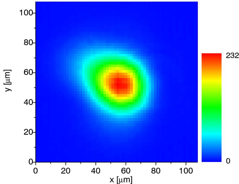
Figure 3.13: Laser beam profile in the focus of a  $f = 300$  mm achromatic lens as measured by the CCD camera imaging system. The image covers  $60 \times 60$  pixels of the CCD camera. The  $1/e^2$  diameter of the beam is  $2w = 59 \mu\text{m}$ .
