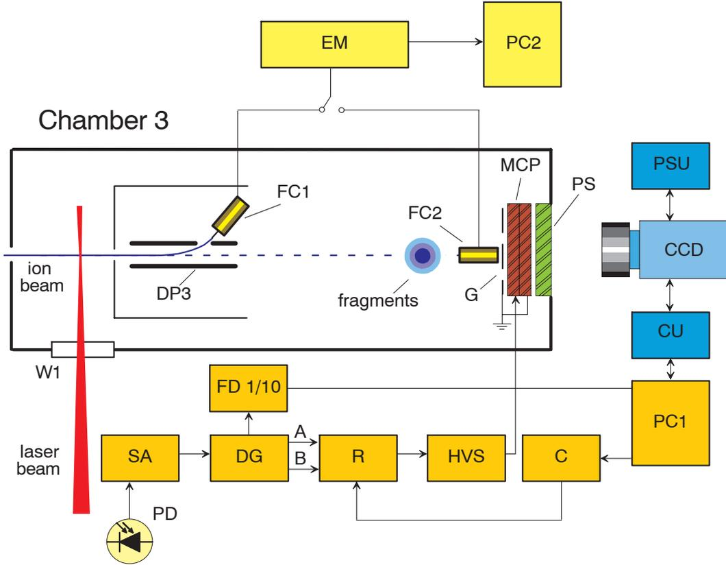
Figure 3.5: Schematic of Chamber 3 and the components used in the detection. W1, window; PD, photodiode; SA, signal amplifier; DG, delay generator; FD, frequency divider; R, relay; HVS, high-voltage switch; C, 2-bit counter; PC, personal computer; CU, CCD control unit; PSU, Peltier stabilization unit; EM, electrometer; DP, deflection plates; FC, Faraday cup; G, grid; MCP, multichannel plate detector; PS, phosphor screen.
