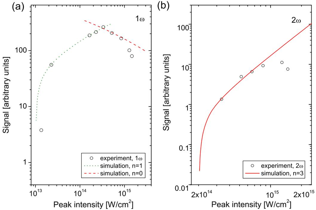
Figure 5.6: The total fragment signal in the (a) one-photon bond softening and (b) net two-photon process as a function of the peak laser intensity. The curves show the results of simulations of a  $I^n$  dependence (see the text).
