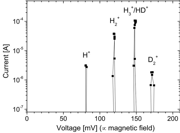
Figure 3.3: Ion current measured at apertures A3 and A4 as a function of the voltage (i.e., magnetic field) on the sector magnet. The ions result from ionization and recombination processes in a  $\text{H}_2$  plasma. The acceleration voltage was  $U_a = 12$  kV.
