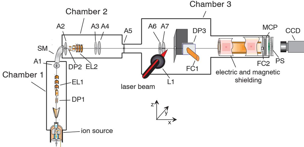
Figure 3.1: Schematic diagram of the ion beam apparatus. DP, deflection plates; EL, Einzel lenses; SM, sector magnet; A, apertures; L1, focusing lens; FC, Faraday cups; MCP, multichannel plate detector; PS, phosphor screen; CCD, CCD (charge-coupled device) camera.
