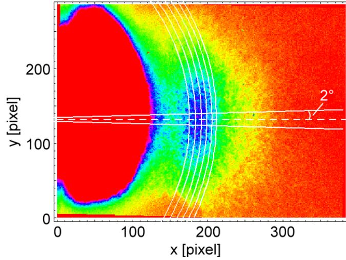
Figure 6.7: Projected 2D velocity distribution of the protons in the Coulomb explosion channel of  $\text{H}_2^+$  at an intensity of  $8.8 \times 10^{13} \text{ W/cm}^2$ . The integration range for the spectra in Fig. 6.6 is indicated by the lines at an angle of  $2^\circ$  with the symmetry axis. The circular arcs mark the position of the main peaks between the kinetic energies of 1.3 and 1.6 eV in Fig. 6.6(a).
