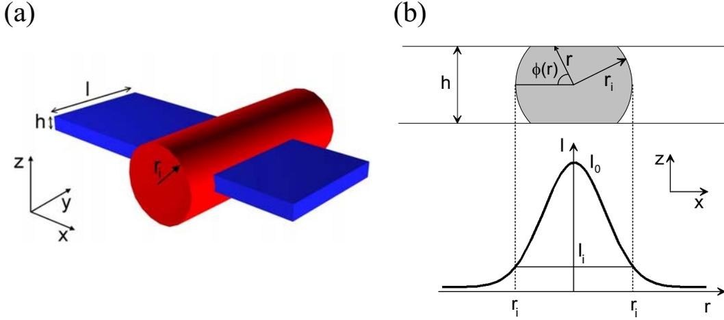
Figure 3.17: (a) Interaction volume defined by the intersection of a laser beam (shown as a cylinder) and an ion beam (box). (b) A cut in the  $x$ - $z$  plane. The shaded area denotes the region with intensities  $I > I_i$ . The intensity distribution along the  $x$  axis is illustrated below.
