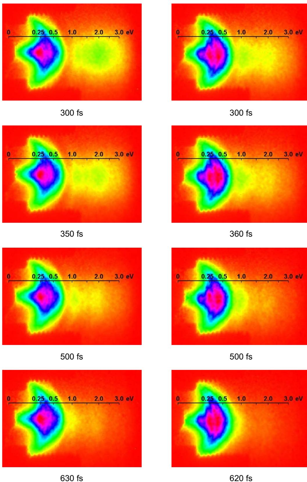
Figure 6.13 (continued): Projected 2D velocity distributions from photodissociation and Coulomb explosion of  $D_2^+$  (left) and  $H_2^+$  (right) for the different pulse durations.
