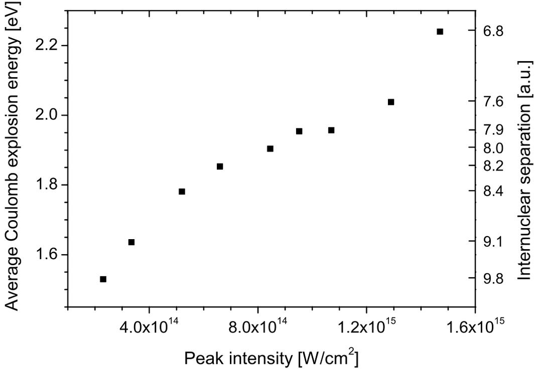
Figure 6.3: Average kinetic energy of the Coulomb explosion protons as a function of the peak laser intensity. The data were derived from the kinetic energy spectra obtained by integrating the inverted velocity distributions in Fig. 5.2 over all angles. The axis on the right side marks the corresponding internuclear separations at which the ionization occurs.
