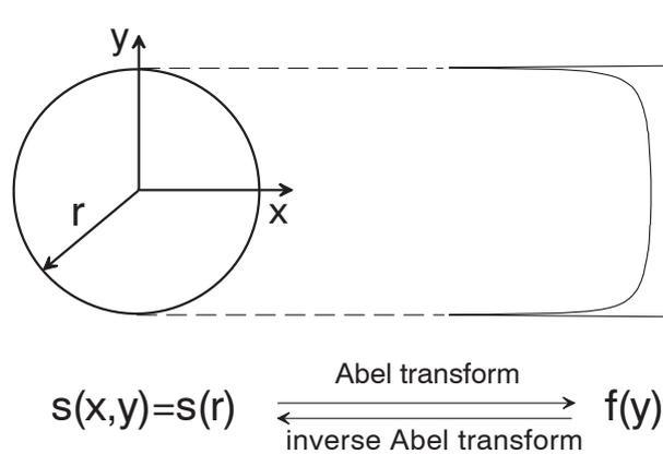
Figure 3.9: The Abel projection of a slice through the 3D velocity distribution at  $z = z_0$  onto the  $y$  axis. The distribution  $s(r)$  on the slice can be retrieved from the projected distribution  $f(y)$  using the inverse Abel transform.
