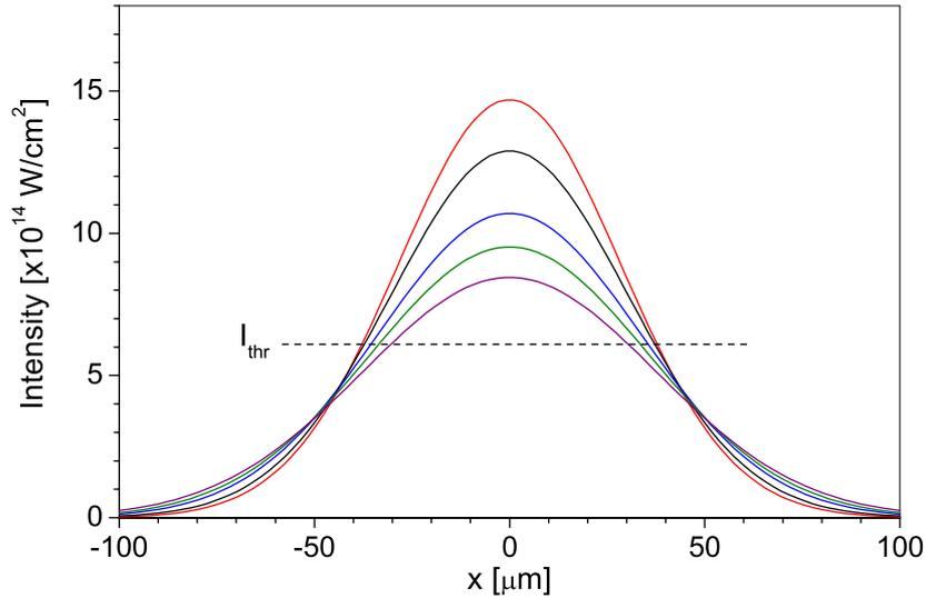
Figure 6.4: Gaussian distributions illustrating one-dimensional spatial intensity distribution for the measurements at highest intensities in Fig. 6.3. The areas under the distributions are the same, corresponding to the same pulse energy, whereas their widths are smaller for higher peak intensities. Only intensities above the threshold intensity  $I_{thr}$  for a particular process contribute to the measured signal.
