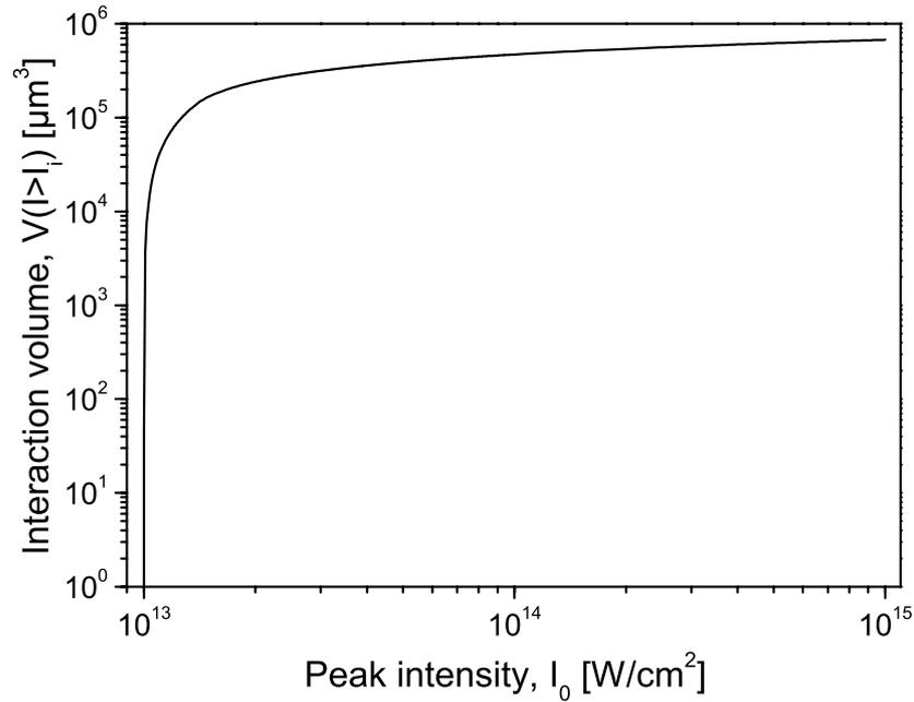
Figure 3.18: Interaction volume  $V(I > I_i)$  as a function of the peak intensity  $I_0$  for threshold intensity  $I_i = 1 \times 10^{13}$  W/cm<sup>2</sup>. The parameters used in the calculation were  $w = 30$   $\mu\text{m}$ ,  $h = 25$   $\mu\text{m}$  and  $l = 300$   $\mu\text{m}$ .
