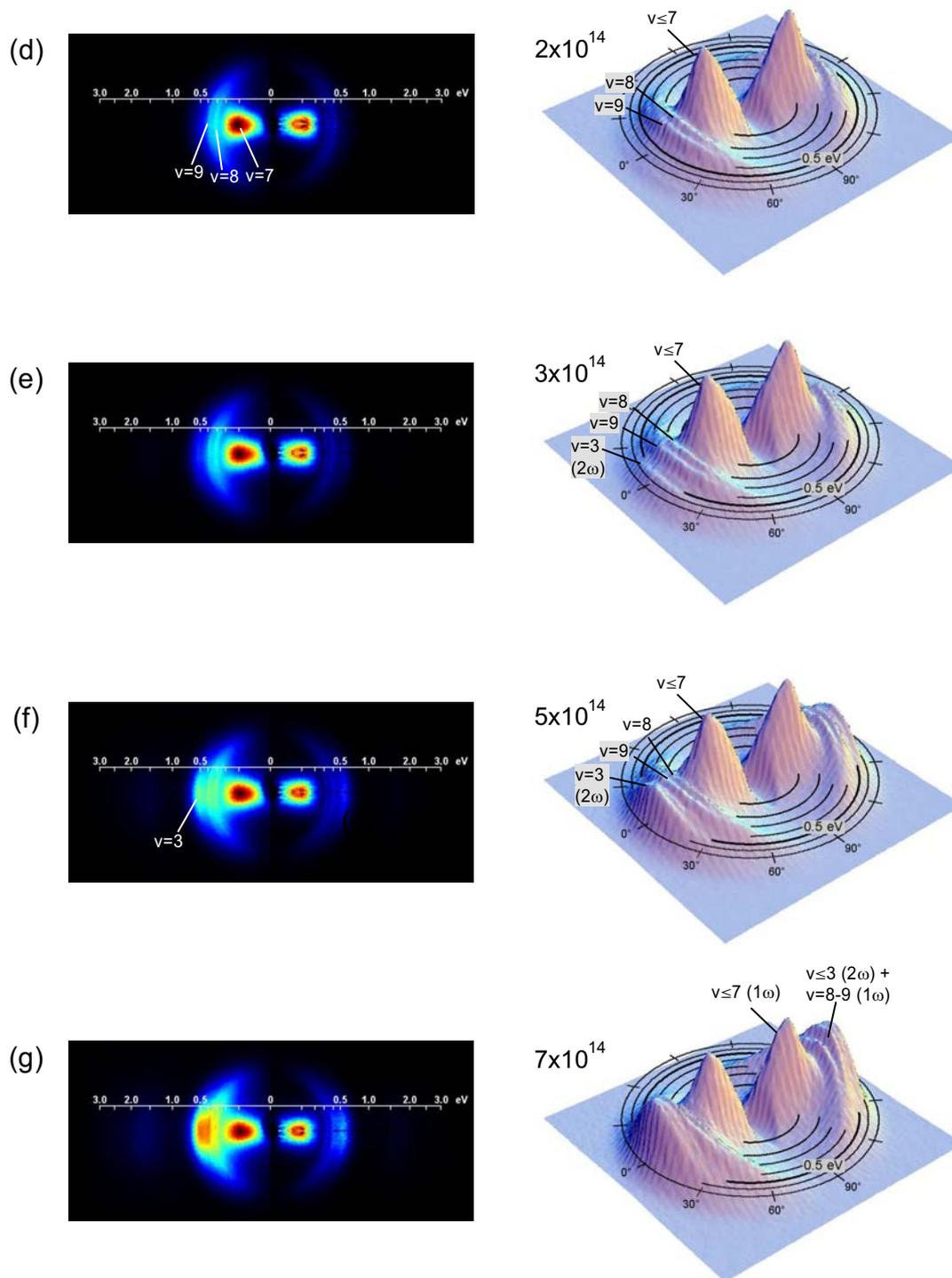
Figure 5.2 (continued): Velocity distributions of the fragments resulting from photodissociation and Coulomb explosion of  $\text{H}_2^+$  at different peak intensities.
