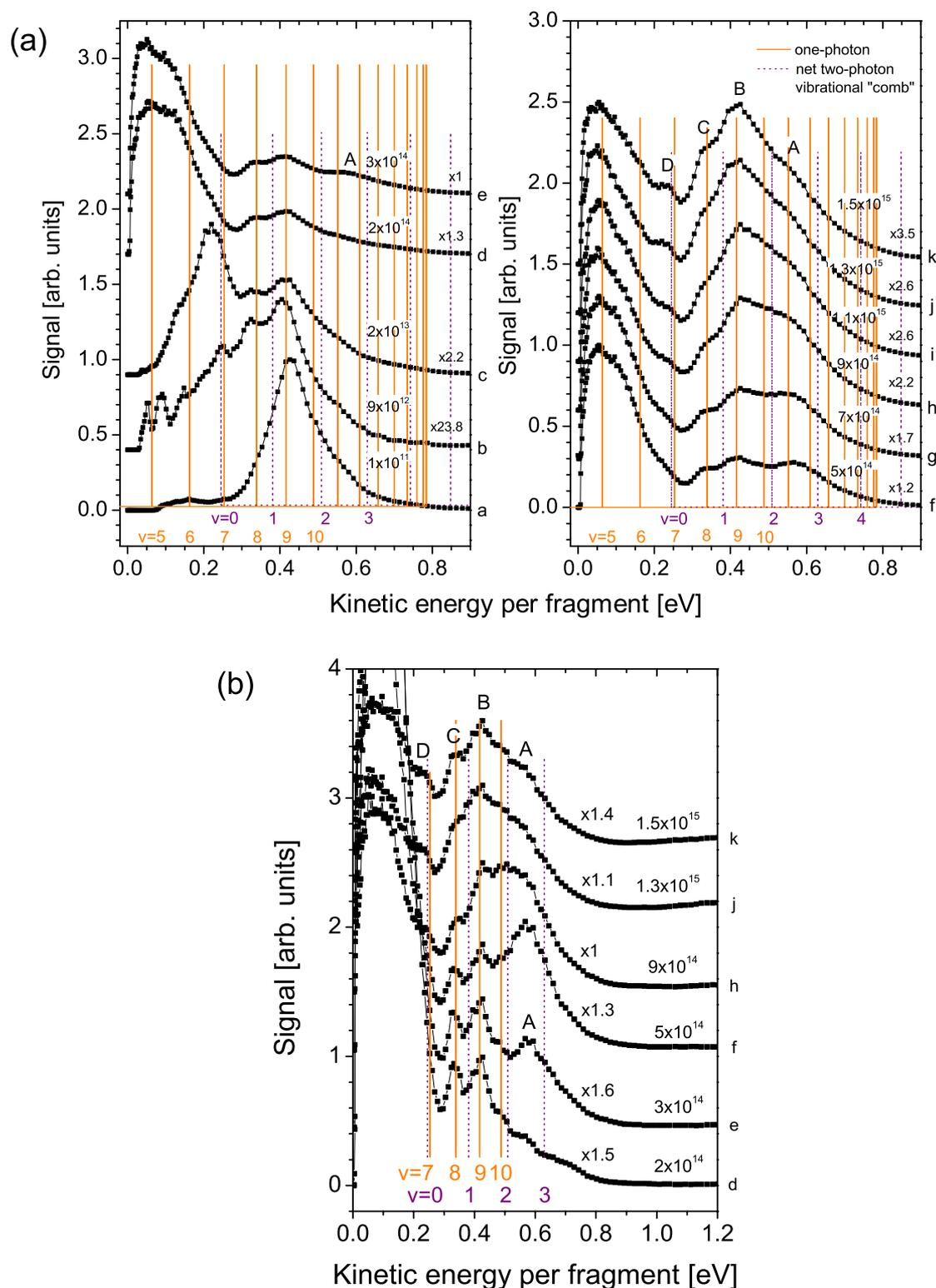
Figure 5.3: Kinetic energy distributions of the fragments obtained by integrating inverted velocity distributions over (a) all angles and (b)  $10^\circ$  around the laser polarization axis. In (b), only the part of the spectra with the net two-photon contribution is shown. The peak laser intensities and the scaling factors are given for each measurement. The measurements are labelled with letters as in Fig. 5.2.
