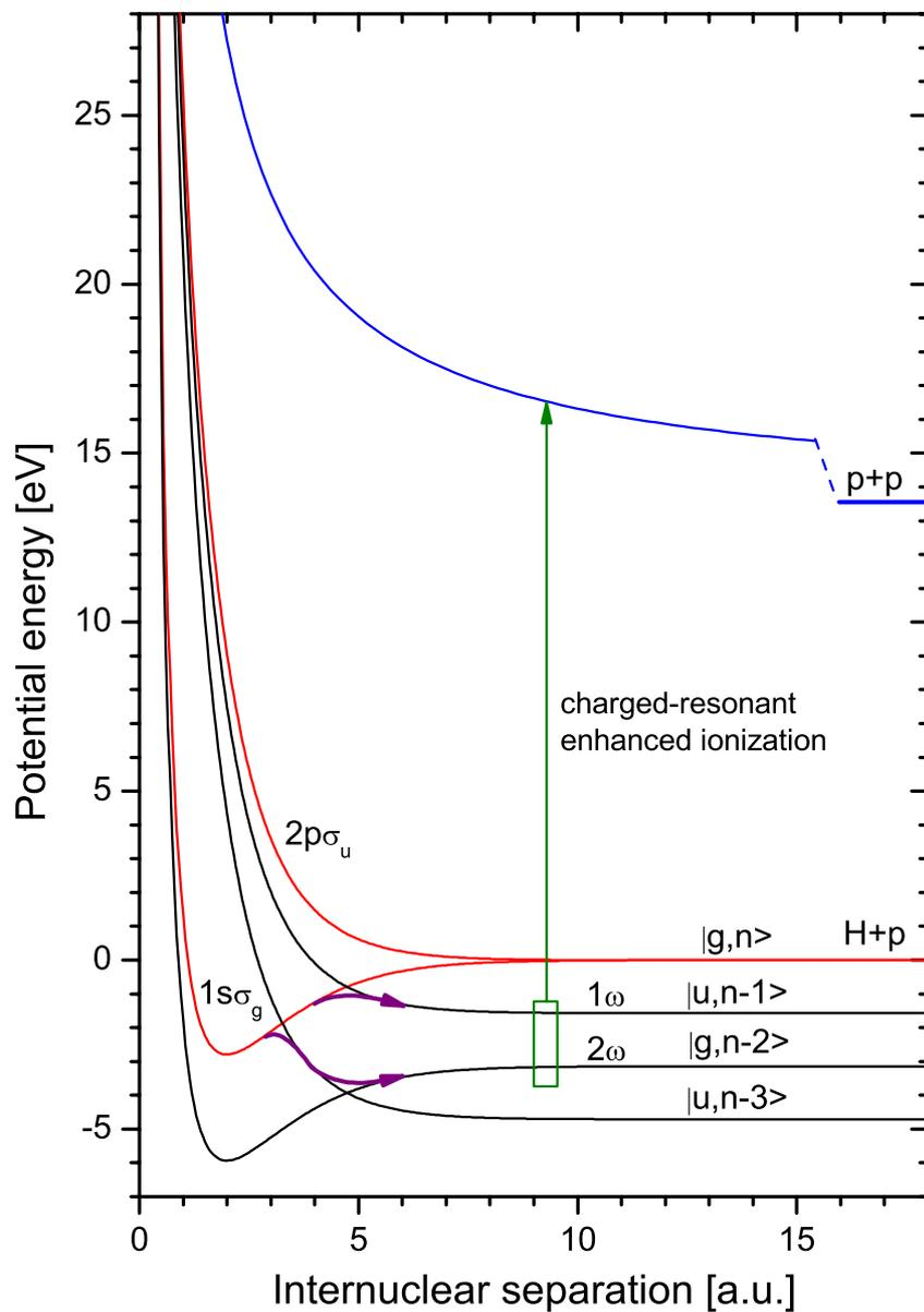
Figure 6.2: Potential energy diagram illustrating the mechanism of Coulomb explosion. The molecules dissociate by following the one- ( $1\omega$ ) or net two-photon ( $2\omega$ ) process. At relatively large internuclear separations, a dissociating molecular ion undergoes ionization and subsequent Coulomb explosion of nuclei. The measured kinetic energy per fragment is thus the sum of the initial dissociation energy and the CE energy.
