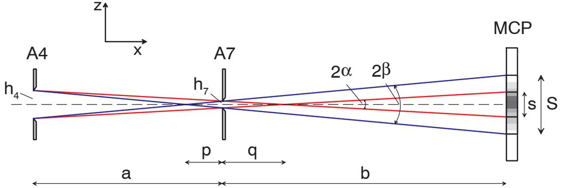
Figure 3.6: Schematic diagram of the geometry employed for collimation along the  $z$  axis. Apertures A4 and A7 are not drawn to scale.
