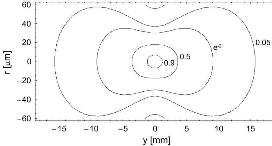
Figure 3.16: Spatial intensity distribution of a Gaussian beam at the focus, described by the axial and radial coordinates. The calculation was made for  $w_0 = 30 \mu\text{m}$  and  $y_R = 3.6 \text{ mm}$ . The labels designate intensities at the contours in units of the maximum peak intensity  $I_f$ .
