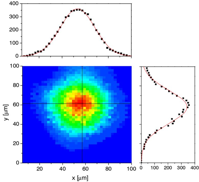
Figure 3.15: The laser beam intensity profile measured in the focus of a  $f = 300$  mm achromatic lens by means of a scanning pinhole followed by a photodiode. The scanning step was  $2.4 \mu\text{m}$  along both axes. The horizontal and vertical profiles were fitted by Gaussian distributions with diameters  $2w_x = 60 \mu\text{m}$  and  $2w_y = 69 \mu\text{m}$ .
