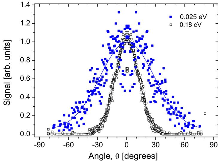
Figure 4.7: Angular distributions from Fig. 4.6 at kinetic energies of 0.025 eV and 0.18 eV (radii of 30 and 80 in Fig. 4.6). Each angular distribution comprises data at five adjacent radii. The solid lines show fits to Gaussian distributions with FWHMs of  $56 \pm 3^\circ$  and  $29.5 \pm 0.2^\circ$ . The corresponding  $\langle \cos^2 \theta \rangle$  parameters are  $0.84 \pm 0.04$  and  $0.954 \pm 0.006$ , respectively.
