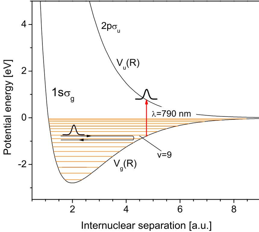
Figure 2.1: The two lowest electronic states of  $H_2^+$  coupled by laser radiation centered at a wavelength of 790 nm. The Franck-Condon factor is maximal for the vibrational level  $v = 9$  at an internuclear separation of 4.8 a.u.
