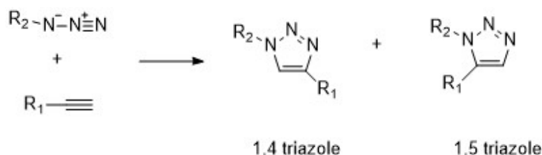
Scheme 1. 3. Huisgen reaction. The reaction between a terminal alkyne and an azide gives a mixture of the two regioisomers 1,4 and 1,5 triazoles.
