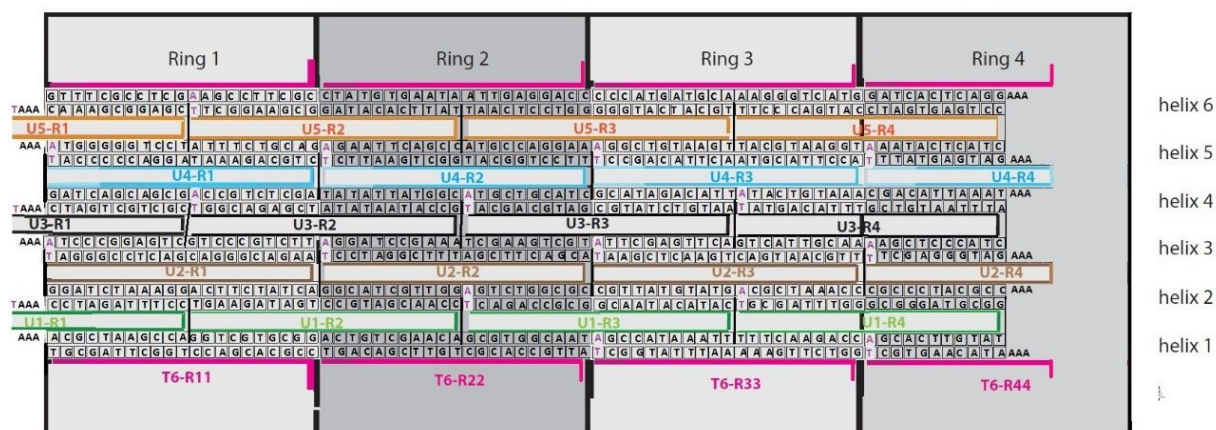
Figure 3. 8. Design of the unmodified tile assembled structure (6HT). [2] The structure has a calculated length of 27 nm and an outer diameter of 8.5 nm. The helices bow slightly outwards due to the electrostatic repulsion between the negatively charged backbones of the DNA.
