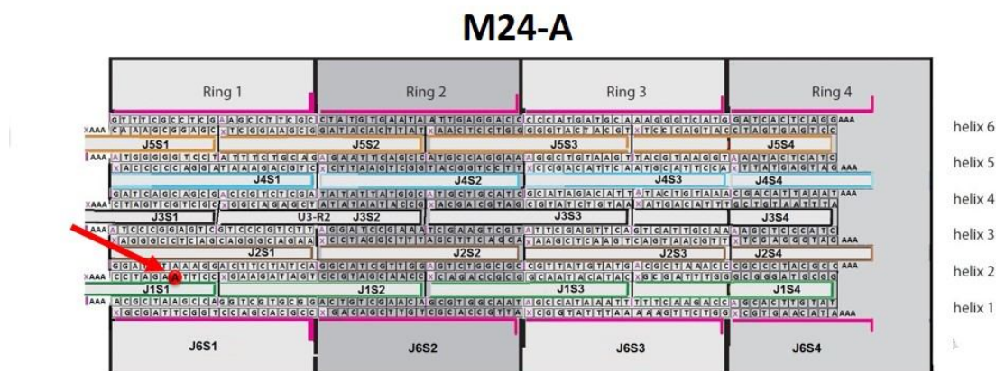
Figure 3. 38. Design of the completely modified tile assembled structure (all 24 strands are azide/alkyne modified) containing the fluo- click -tile V1C1 (M24-A). The red dot corresponds to the fluorescent labelled position.
