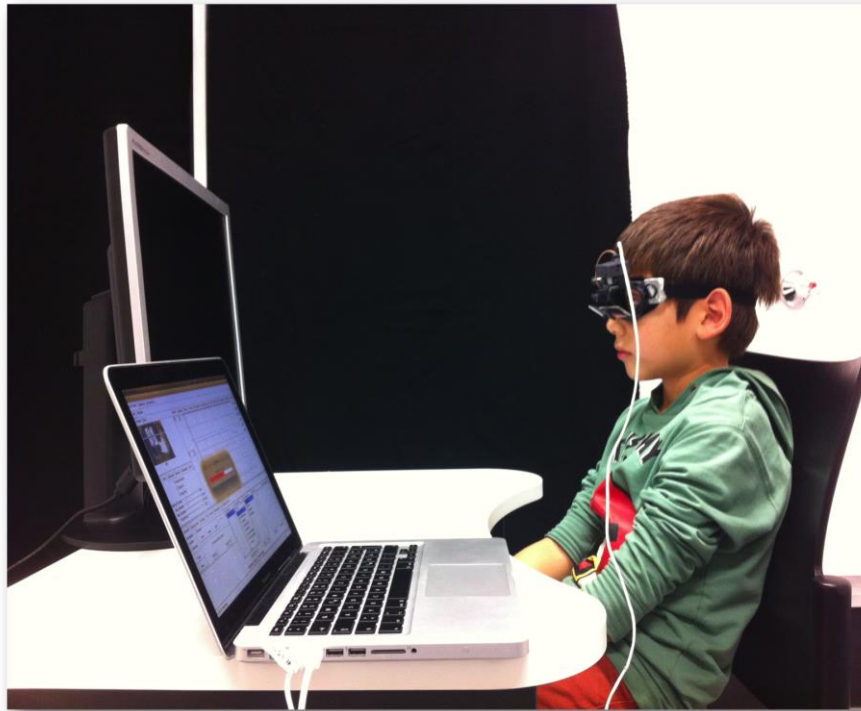
Figure 6. Mobile video-oculographic set-up allows non-invasive measurement of pediatric patients.
