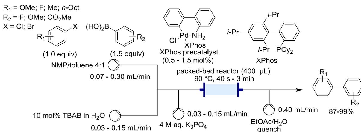
**Scheme 15:** *Suzuki-Miyaura* cross-couplings in a flow reactor.<sup>60</sup>
