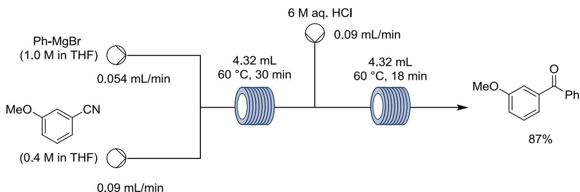
**Scheme 13:** Continuous flow synthesis of ketones by addition of *Grignard* reagents to nitriles with subsequent imine hydrolysis.<sup>56</sup>
