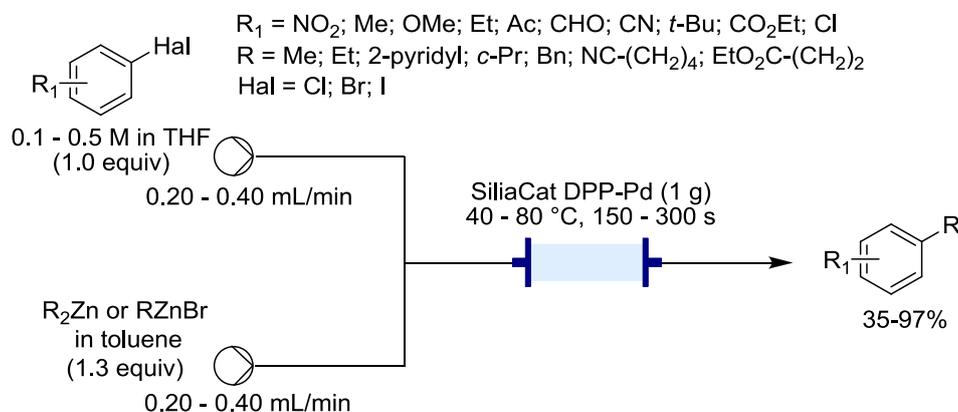
**Scheme 17:** First alkyl-aryl *Negishi* cross-couplings in a continuous flow reactor.<sup>66</sup>
