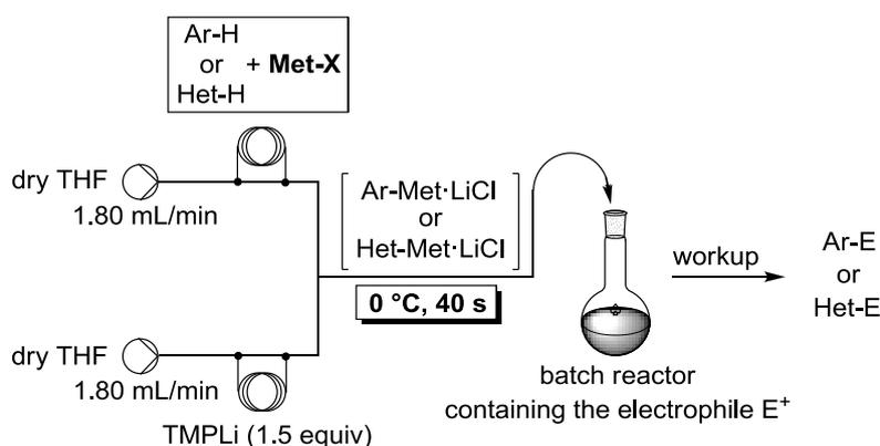
**Scheme 25:** Continuous flow set-up for *in situ* trapping metalations using TMPLi in the presence of metal salts (Met-X =  $\text{ZnCl}_2 \cdot 2\text{LiCl}$ ,  $\text{MgCl}_2$ ,  $\text{CuCN} \cdot 2\text{LiCl}$ ,  $\text{LaCl}_3 \cdot 2\text{LiCl}$ ) and subsequent batch quenching with electrophiles ( $\text{E}^+$ ).
