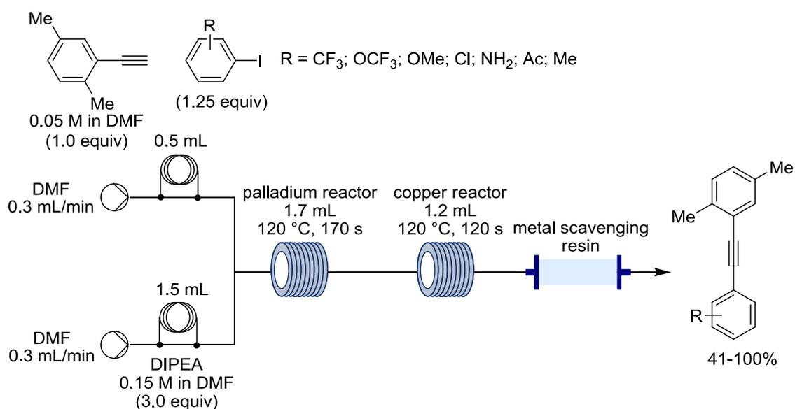
**Scheme 16:** Heterogeneous *Sonogashira* cross-coupling in a palladium-copper dual flow reactor. Yields were determined by GC-analysis.<sup>63</sup>
