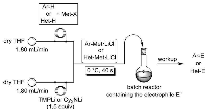
**Scheme 29:** Continuous flow set-up for *in situ* trapping metalations using TMPLi or  $\text{Cy}_2\text{NLi}$  in the presence of metal salts (Met-X =  $\text{ZnCl}_2\cdot 2\text{LiCl}$ ,  $\text{MgCl}_2$ ,  $\text{CuCN}\cdot 2\text{LiCl}$ ,  $\text{LaCl}_3\cdot 2\text{LiCl}$ ) and subsequent batch quenching with electrophiles ( $\text{E}^+$ ).
