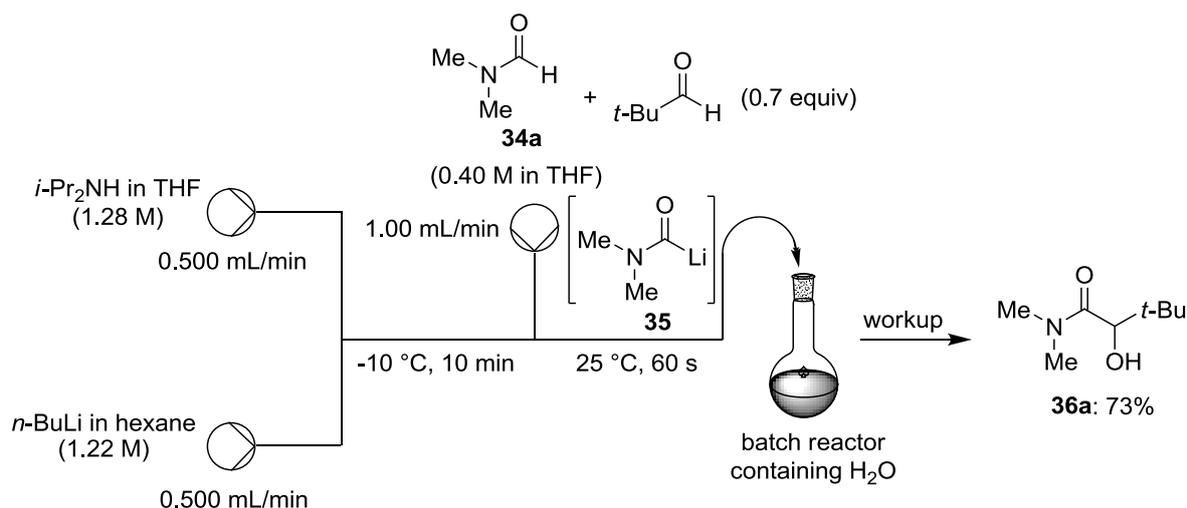
**Scheme 35:** Continuous flow set-up for the *in situ* trapping metalation of dimethylformamide (**34a**) using LDA in the presence of trimethylacetaldehyde.
