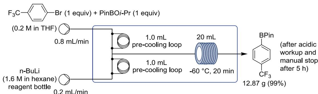
**Scheme 14:** Multi-gram synthesis of arylboronic acid pinacol esters using a novel cryostatic flow reactor.<sup>59</sup>
