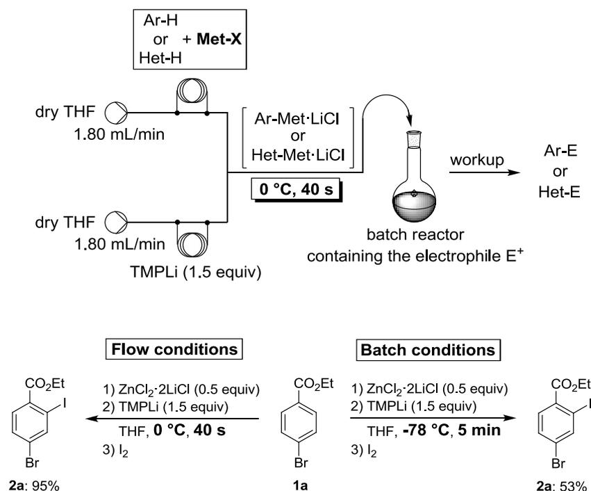
**Scheme 23:** Continuous flow set-up for *in situ* trapping metalations using TMPLi in the presence of metal salts (Met-X = ZnCl<sub>2</sub>·2LiCl, MgCl<sub>2</sub>, CuCN·2LiCl, LaCl<sub>3</sub>·2LiCl) (top) and iodination of ethyl 4-bromobenzoate (**1a**) using flow and batch conditions for the *in situ* trapping metalation (bottom).
