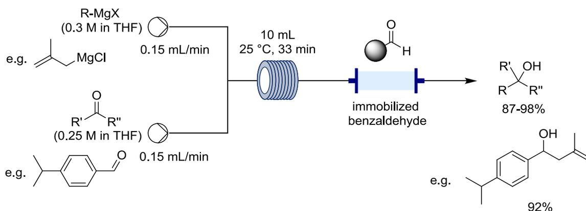
**Scheme 12:** Reaction set-up for the addition of organomagnesium reagents to carbonyl compounds to form secondary and tertiary alcohols. The immobilized benzaldehyde was utilized for scavenging unreacted *Grignard* reagent.<sup>55</sup>
