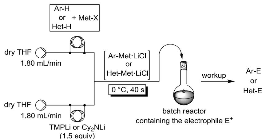
**Scheme 34:** Continuous flow set-up for *in situ* trapping metalations using TMPLi or  $\text{Cy}_2\text{NLi}$  in the presence of metal salts (Met-X =  $\text{ZnCl}_2\cdot 2\text{LiCl}$ ,  $\text{MgCl}_2$ ,  $\text{CuCN}\cdot 2\text{LiCl}$ ,  $\text{LaCl}_3\cdot 2\text{LiCl}$ ) and subsequent batch quenching with electrophiles ( $\text{E}^+$ ).
