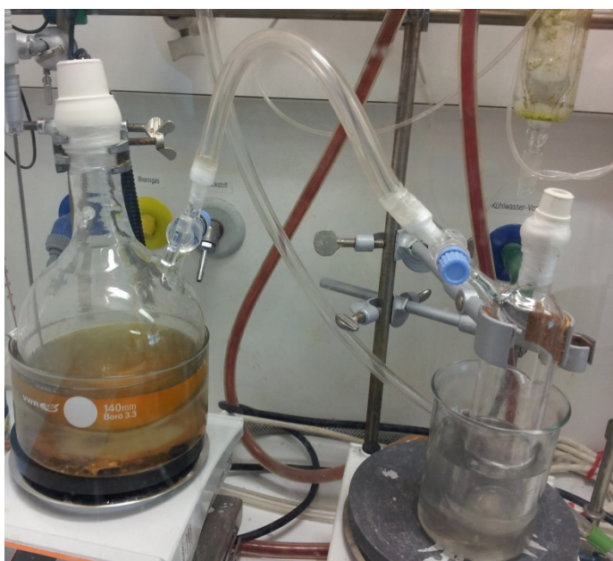
Figure S1. Experimental set up for the synthesis of AB-component 12 . For safety reasons the whole experimental set up is assembled behind a blast shield. The left reaction chamber contains a suspension of tetrakis(triphenylphosphine)palladium(0), triflate 25 , lithium chloride and tributylamine in acetonitrile. A rubber tube connects this chamber to a second Schlenk flask containing sulfuric acid and formic acid for carbon monoxide generation.
