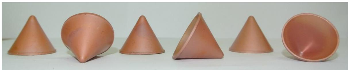
**Figure 2.** Liners made from copper (ECu) powder.
