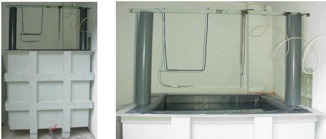
**Figure 6.** The arrangement for the underwater explosion tests (left) and the positioning system with the sensor and detonator (right).
