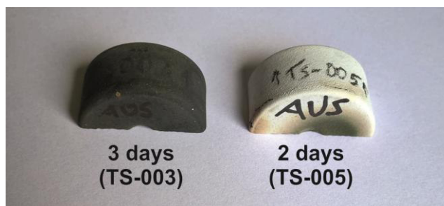
Fig. 4-4: Photographs showing the samples treated for two (TS-005) and three (TS-003) days. The samples are cut by half. Sample diameter is 2 cm.
