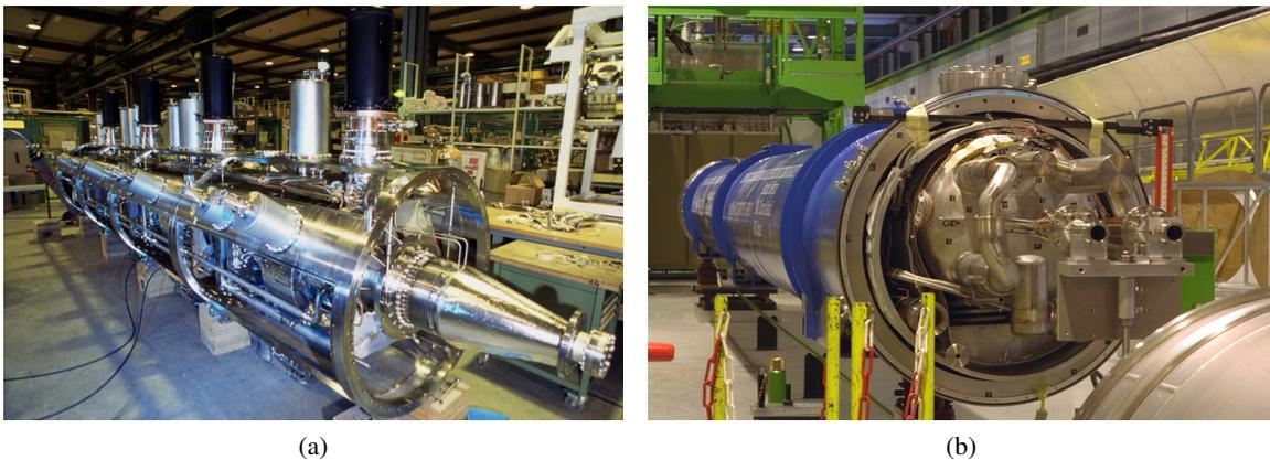
Figure 3.2.: Pictures of a RF cavity (Fig. (a)) and a dipole magnet (Fig. (b)) prior to their installation in the LHC tunnel [43, 44].
