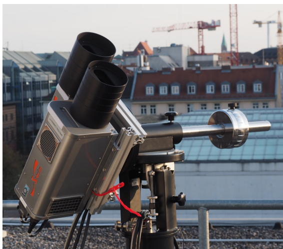
Figure 5.1: specMACS VNIR and SWIR sensors on scanning mount. The stray light protection is prominently visible in front of the sensors.
