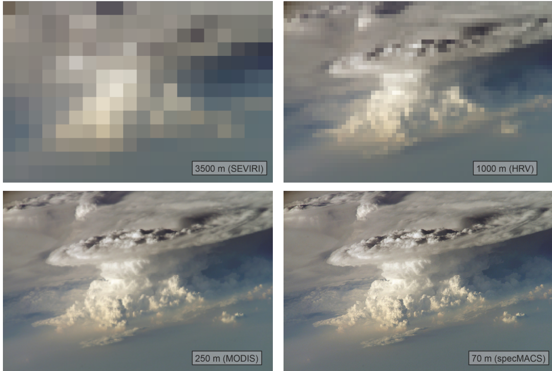
Figure 1.2: Influence of spatial resolution \Delta x of a cloud side as it would be measured (a) by the geostationary imager SEVIRI ( \Delta x = 3500 m), (b) by its High Resolution Visible (HRV) channel ( \Delta x = 1000 m), (c) by the Earth-orbiting imager MODIS ( \Delta x = 250 m) and (d) by the specMACS instrument ( \Delta x = 70 m) which was developed during this thesis. Original picture: Thunderstorm Off the Coast of Republica de Chile (taken from the International Space Station), ISS015-E-27038, September 7, 2007.
