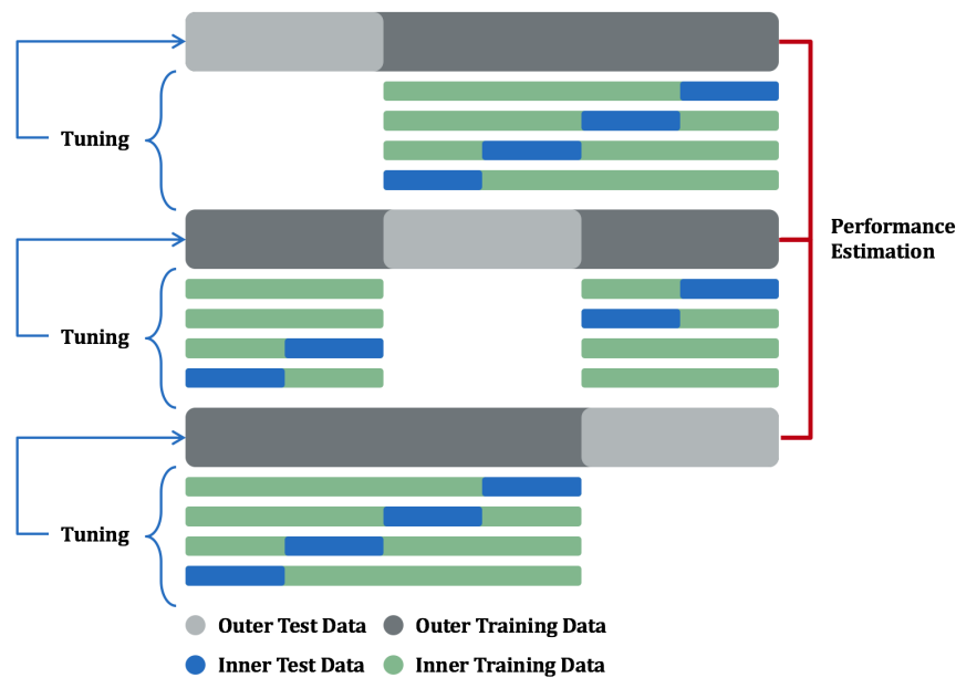
Figure 1.6: Nested Resampling; hyperparameter tuning is performed in the respective inner resampling iteration (4-fold CV), tuned parameters used for model evaluation in the respective outer iteration (3-fold CV), mean predictive performance is calculated across all outer resampling iterations.
