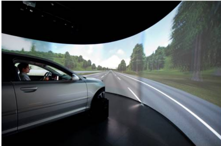
Figure 2.1: Driving simulator apparatus and car mockup at AUDI headquarters in Ingolstadt, Germany. Picture, as courtesy by the AUDI AG.
