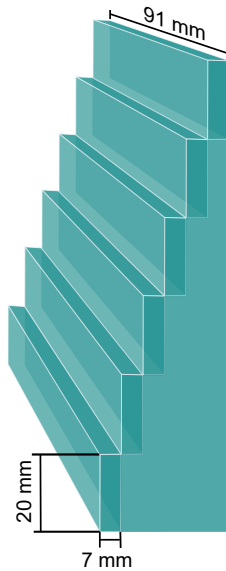
Figure 3.38: Homogeneous PMMA stepped-wedge phantom used for radiographic investigations.
