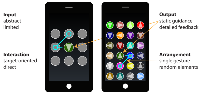
Figure 4.13: Connect four is a modification of pattern rotation which is based on randomized input elements and a secret cue. During enrollment, the system displays a specific color and a direction (left). During authentication, the user recognizes the assigned color (right).
