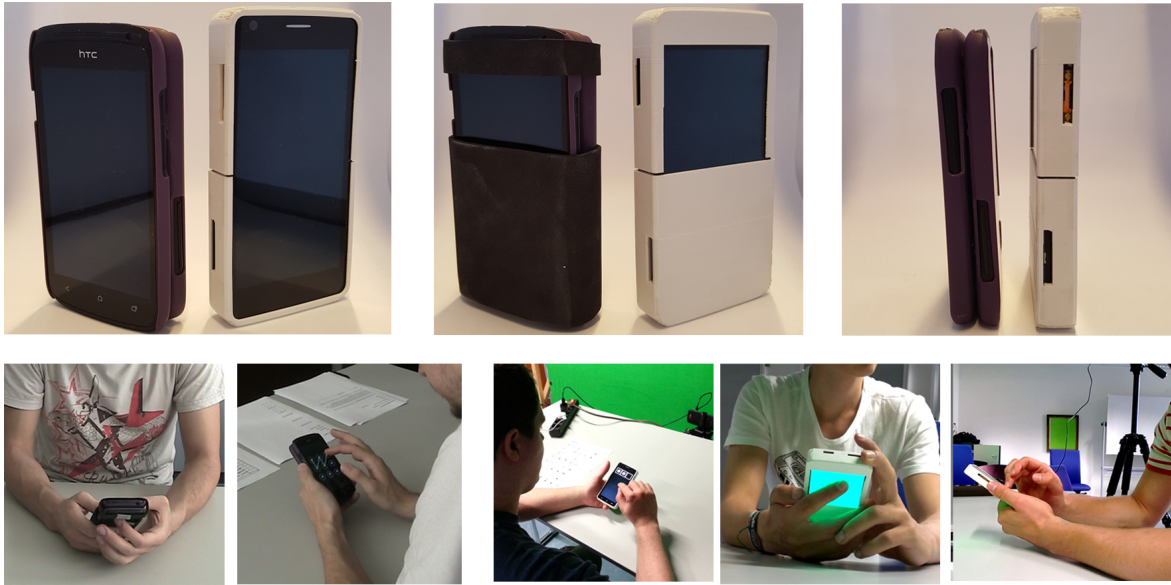
Figure 4.30: The first row shows two XSide prototypes with the white prototype being the improved version. The lower row illustrates the camera setup used for the observation attacks. The two images on the left originate from the first user study, the three pictures on the right show participants of the second study.
