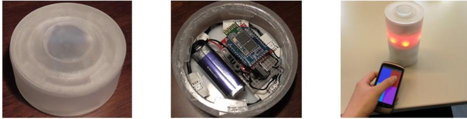
**Figure 7.3: Light cylinders.** The cylinders were built of semi-transparent acrylic and equipped with an Arduino board and LEDs. Colors of individual cylinders are changed via a smartphone app.
