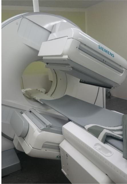
Figure 1.3: Image of a Siemens Symbia Intevo T16 SPECT/CT during a rotation around the camera table
