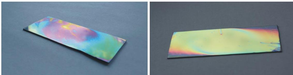
**Figure 2.** Photographs of 3-bilayer Bragg stack 1 (left) and Bragg stack 2 (right) on a  $5 \times 2.5 \text{ cm}^2$  Si substrate in air.
