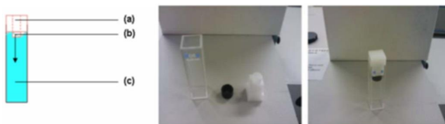
Figure 5.12: Custom made release experiment setup featuring a 200 \mu\text{L} Teflon tube (a) which is closed by a dialysis membrane (b). This setup is put onto a fluorescence cuvette filled with the desired buffer (c).
