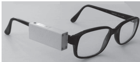
Fig. 15. The LightWatcher: Device for measuring spectral composition of light at the eye level fixed at a spectacle frame.
