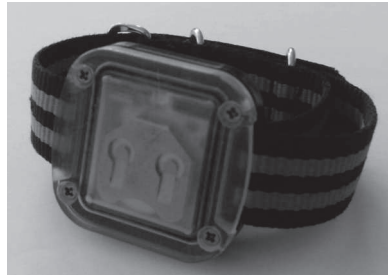
Fig. 14. The Daqtometer®: Wrist worn device for continuous measurement of locomotor activity.
