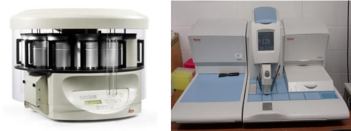
**Figure 9:** Automatic tissue processor (Left) (Adopted from <http://www.leicabiosystems.com>) and embedding apparatus (right) (Adapted from Yildirim Lab).
