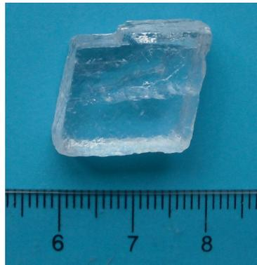
Figure 3.1 Iceland spar crystal that was used to prepare TEM samples.
