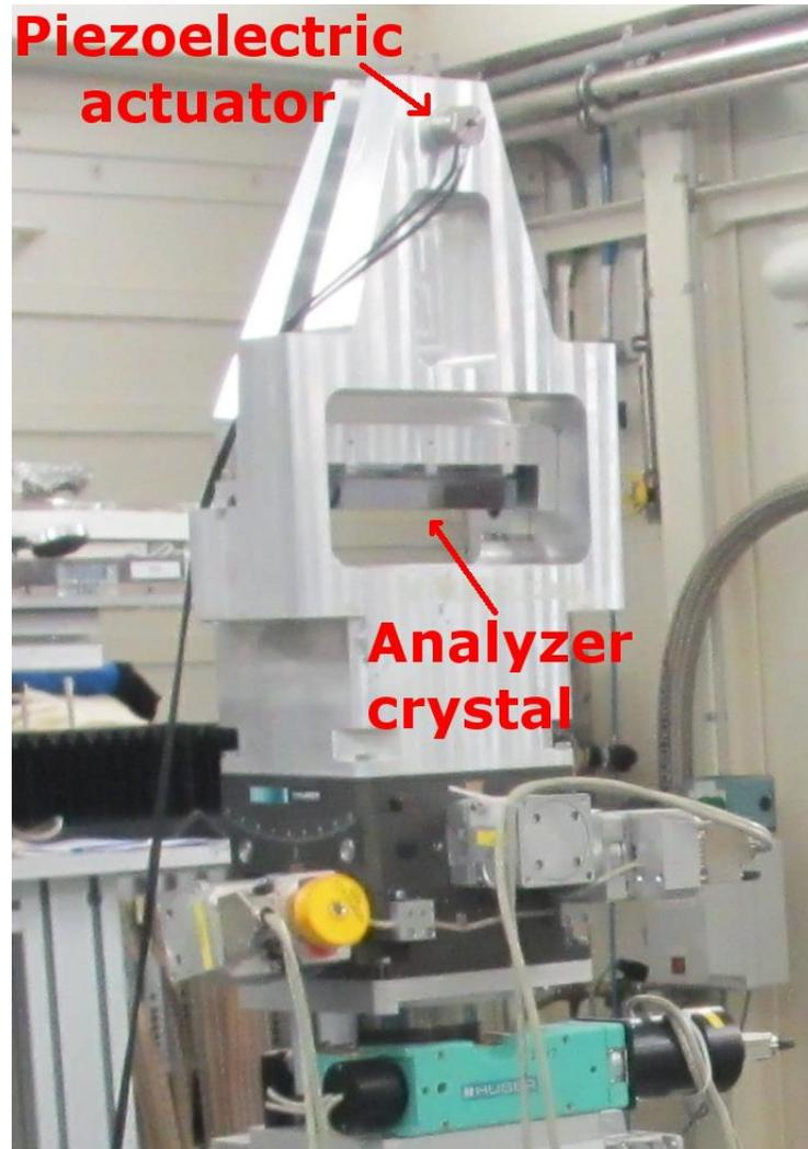
**Figure 2.7:** The analyser stage.
