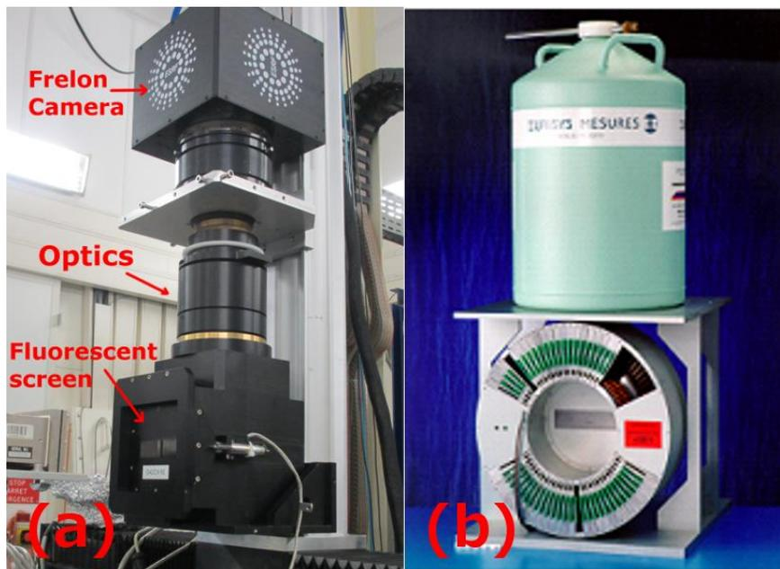
**Figure 2.8:** (a) The ID17 taper optics FReLoN camera; (b) ID17 Germanium detector.
