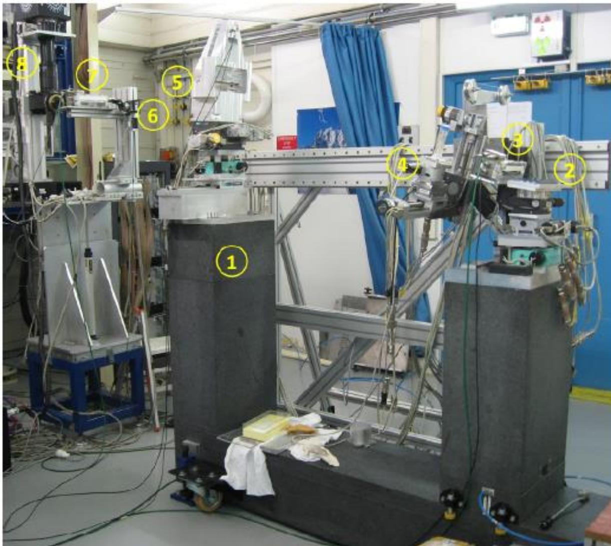
**Figure 2.5:** overview of the setup: (1) granite block; (2) monochromator crystal stage; (3) first ionization chamber; (4) sample stage; (5) analyser crystal stage; (6) diode; (7) second ionization chamber; (8) imaging detector system. Image from Diemoz 2011.
