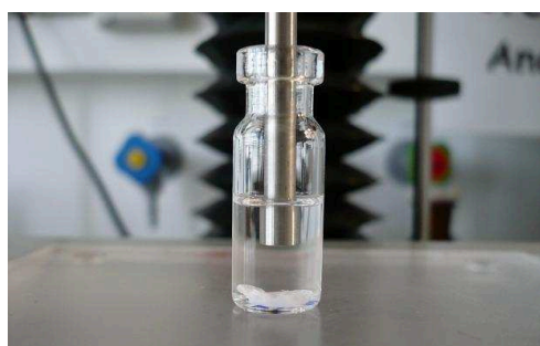
Figure 2-1 Mechanical stress model for simulation of IA conditions during mAb release. After injection of 50 mg of the PLGA formulation a punching tool penetrates into the in situ formed matrix with 20 indentation cycles.
