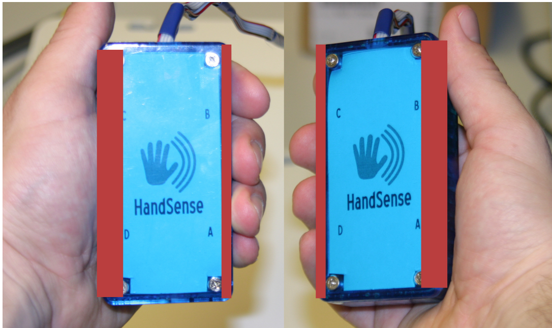
Figure 5.6: HandSense is capable of distinguishing between left-handed and right-handed grasps, even if all sensors are completely covered. The high sensitivity of the capacitive sensors allows to infer the thickness of the tissue in contact with the sensor, thus distinguishing between fingers and palm.
