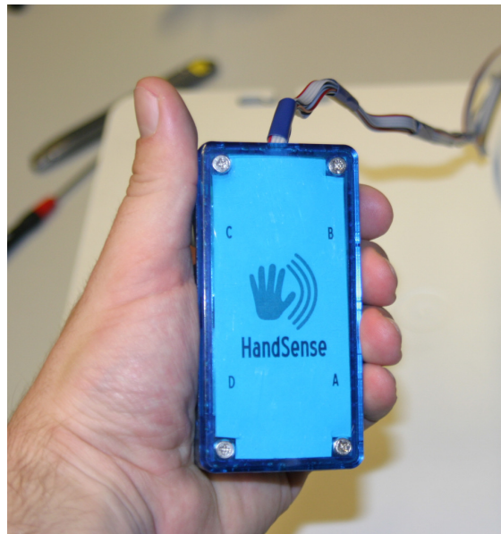
Figure 5.1: The HandSense prototype employs four capacitive proximity sensors - two on each long side. Using heuristics for grasp classification, it allows distinguishing between six different left-handed and right-handed grasps with an average accuracy of 81%.
