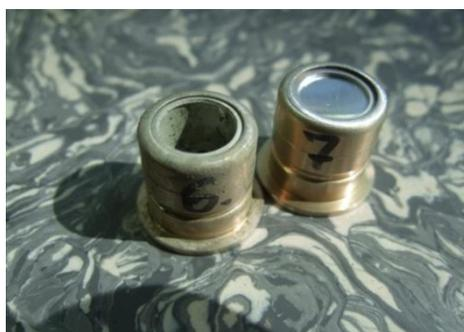
Figure 10. DM 82 burnt down and new.
