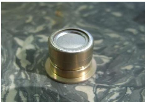
Figure 6. Impulse cartridge DM 82.
