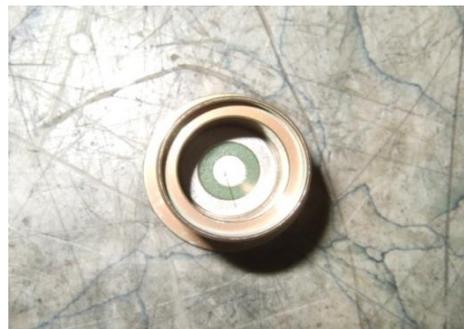
Figure 7. Contacts and bridge wire of the impulse cartridge.
