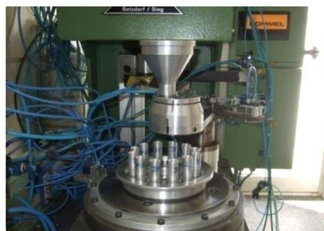
Figure 9. Electronic rotary disc loader.
