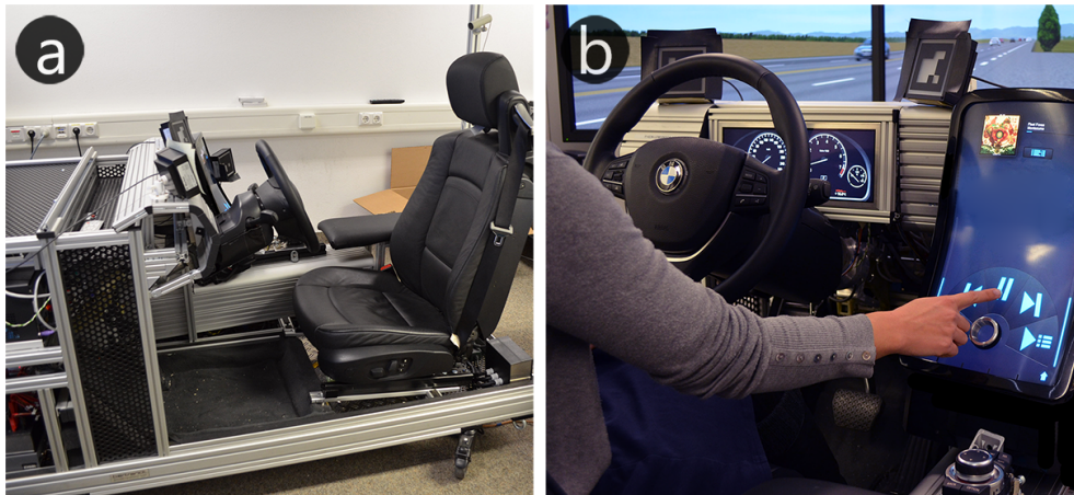
Figure 4.4: Simulator setup for the SimplePlayer evaluation. a: Mock-up b: Visualization of KnobTouch on the 17" touchscreen. Below, the iDrive controller for RemoteControl is attached.
