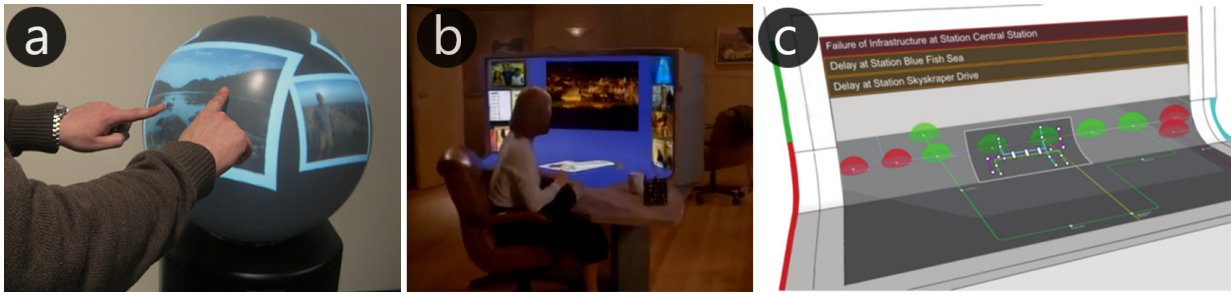
Figure 3.14: Enhancing displayed content by surface shape. a: 3D data on the three-dimensionally shaped Sphere [22] b: StarFire [282] c: Curve with perspective+detail [258].
