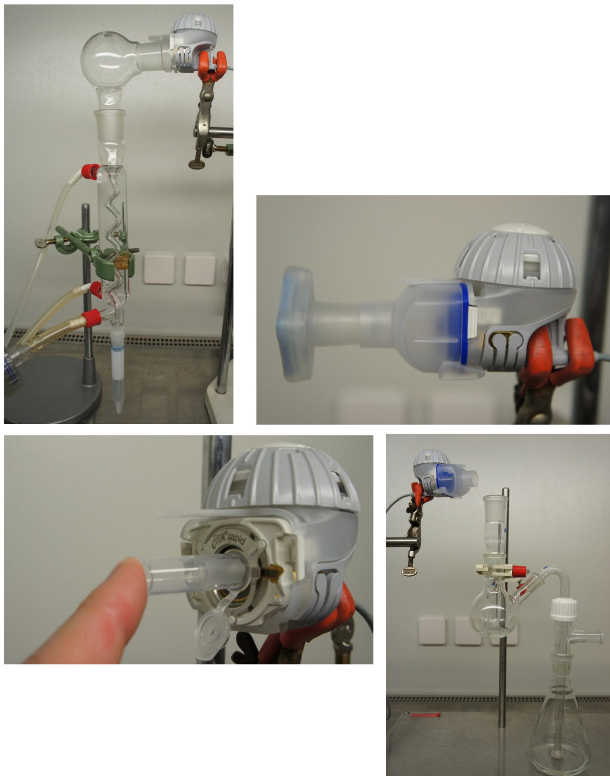
Figure III-4: Pictures of the evaluated aerosol collection methods, including collection in a reflux condenser (top left), in a buffer filled twin-stage impinger (bottom right), inside the aerosol chamber of the nebulizer (top right) or in test tubes (bottom left).
