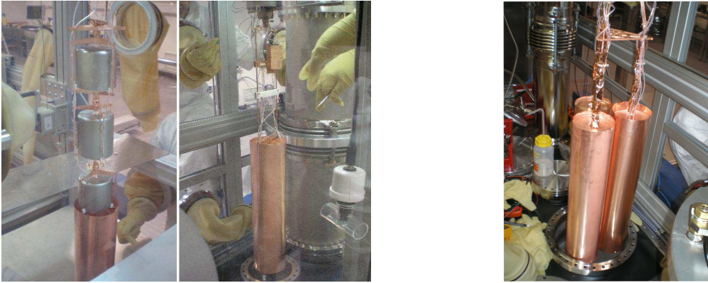
Figure 2.3: GERDA strings with Phase I detectors (on the left) [27] and a mini-shroud (on the right) with a 60\ \mu\text{m} Cu foil jacket for shielding [28].
