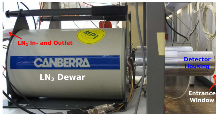
Figure 5.2: Canberra dewar with the REGe detector, mounted inside the aluminium housing.
