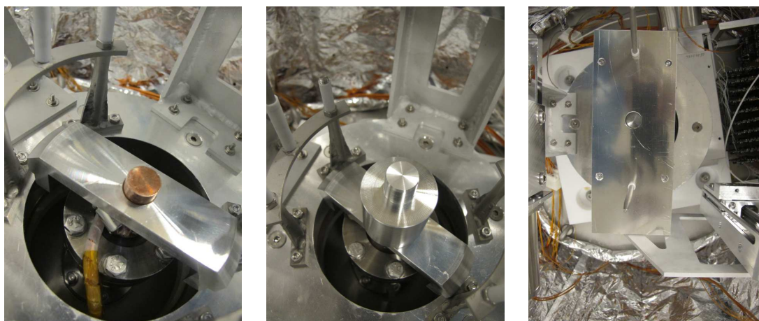
Figure 10.19: Left: tool 1: rounded bail; middle: tool 2: cylinder; right: tool 3: plate used for the detector alignment within the stage.
