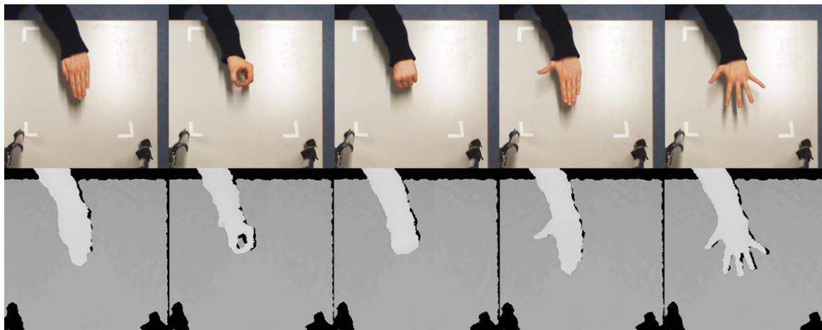
**Figure 8.14:** The five selection gestures (from left to right: *Dwell Time*, *Pinch*, *Fist*, *Thumb* and *Fingers*) and their corresponding depths image (contrast enhanced).
