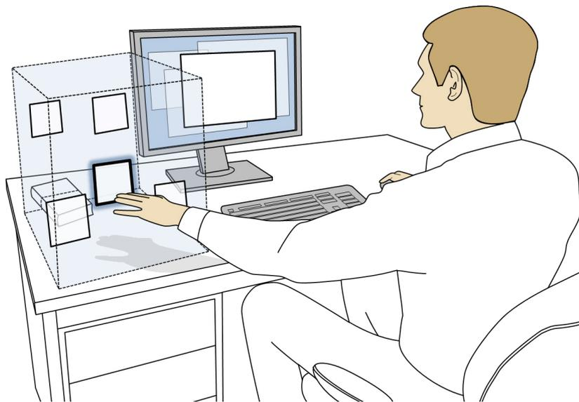
**Figure 8.10:** The Unadorned Desk 3D offers a storage space for virtual items (e.g., commands or applications) left (and/or right). Through a distinct selection gesture, items are placed and retrieved.
