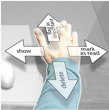
**Figure 7.10:** Four directions for four commands related to emails
