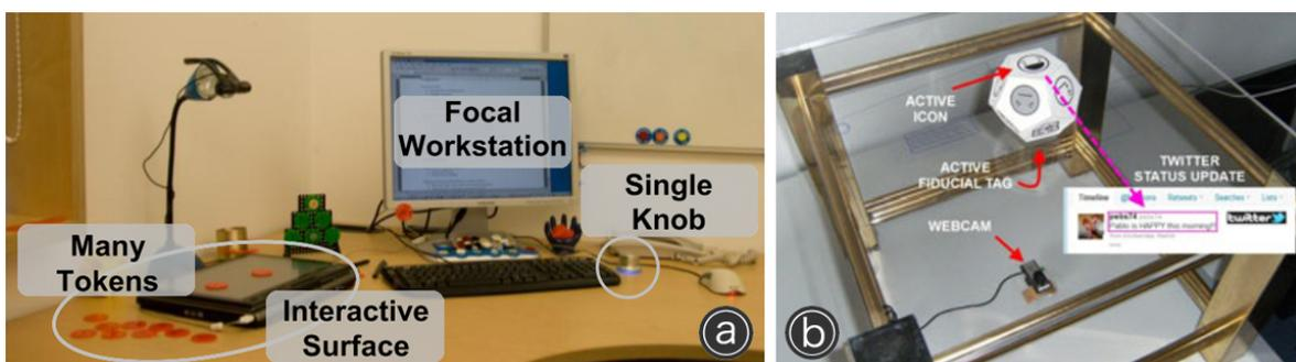
**Figure 4.6:** (a) Task Management System [70], operated bimanually with the tokens on the interactive surface and the knob; and (b) PolyTags [189], used to post updates to a social network or to control an intelligent environment by turning the multi-faced dice.
