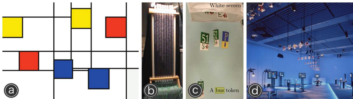
**Figure 4.3:** (a) Informative Art [118], showing the temperature of six cities depicted by squares (position is based on the location on a world map); (b) the Information Percolator [111], rendering images through air bubbles; (c) Bus Mobile [161], displaying nearby buses; and (d) Pinwheels [129], a large scale installation visualizing network traffic.
