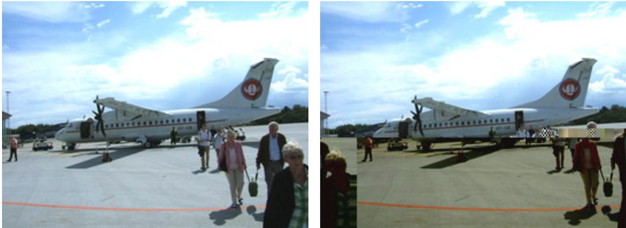
Figure 1.2: Image corruption caused by 1 out of 28466 bytes missing from the file.
