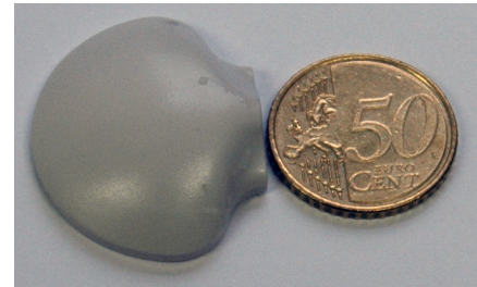
Fig. 2.2.2-2: Transmitter shown with a 50 cent Euro coin (24.25 mm diameter) for size comparison.
