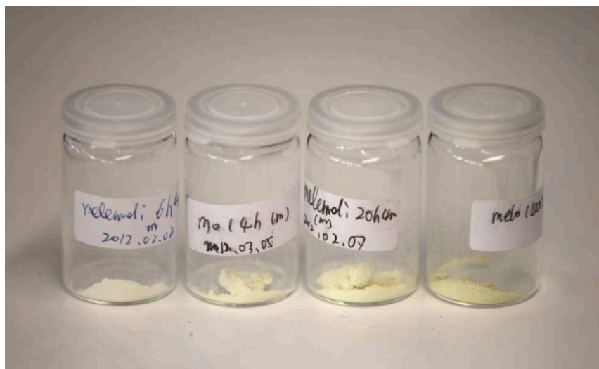
Fig. A.1 Melem oligomers were prepared at 450 °C in open system for 6, 14, 20 and 100 h.
