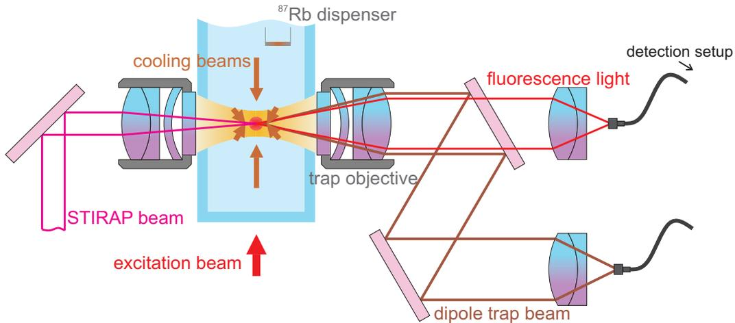
Figure 2.5.: Schematic of the trap setup. It shows the position of both microscope objectives relative to the glass cell which is attached to the UHV-chamber. It also shows the propagation axes of cooling (repump), dipole trap, atomic state readout (STIRAP) and excitation beams.
