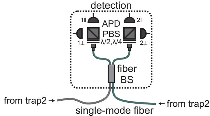
Figure 2.6.: Schematic of the detection setup. It shows the arrangement of the APDs and the polarization analysis as well as the fiber beam-splitter which later combines the light of both experiments.
