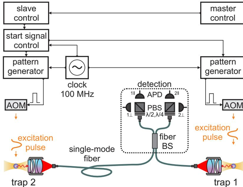
Figure 4.8.: Synchronized experimental setup: The scheme shows the master control which processes the counts from the detectors and controls the slave control. The start signal control switches both pattern generators synchronously into the “experimental pattern”, thus the two single photons impinge on the beam splitter at the same time.
