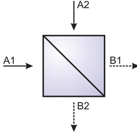
Figure 4.1.: Basic illustration of a beam splitter with two input ports (A1,A2) and two output ports (B1,B2).
