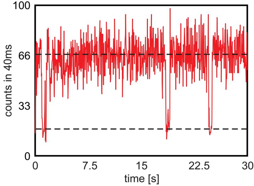
Figure 2.7.: Integrated count rate of single photon detectors. The average detector count rate is  $\sim 1700 \text{ counts/s}$ , if an atom is in the trap. There is a background count rate of  $\sim 400 \text{ counts/s}$ , if no atom is in the trap. The background count rate is caused mainly by reflections of the cooling beams on the glass cell. The graph demonstrates also the fast reloading, if an atom was lost and a long storage time of the atom inside the trap.
