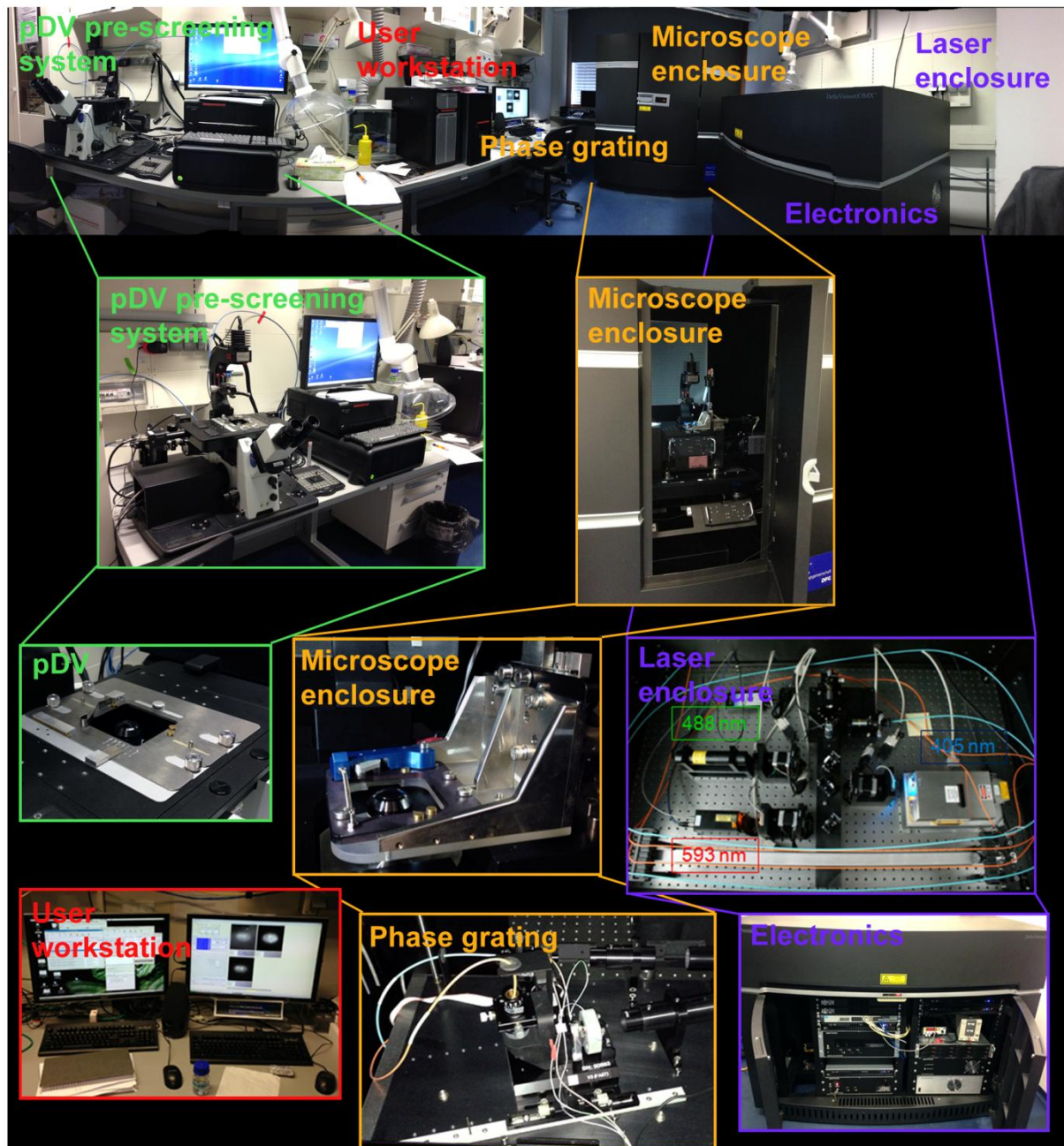
Figure 3-5 OMX V3 prototype setup. The OMX V3 prototype system consists of several components including a conventional pDV wide-field system (green), whose stage is calibrated to the OMX stage allowing eye-piece sample pre-screening in order to collect certain regions of interest within the sample and to visually judge sample quality. The actual OMX V3 3D-SIM system is located within an insulated microscope enclosure (yellow), which also contains the mechanical phase grating device generating the structured illumination pattern. Laser lines are mounted on an open table within a separate laser enclosure (purple), also harboring all electronic equipment necessary for hardware control. Laser enclosure and microscope enclosure are only connected via two multimode laser optical fiber cables separately conducting the SI and the wide-field light path. Super-resolution information gets reconstructed from the SI raw data, channel-aligned and stored on the high-performance user workstation (red) using build-in algorithms of the commercial SoftWorx 4.0 software.
