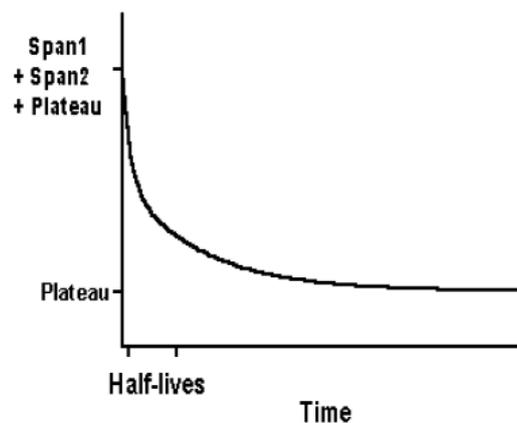
**Figure 8:** Representation two phase regression curve
