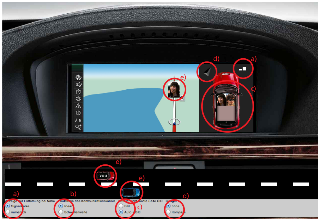
Figure 5.3: Mock-up from the design case of CliqueTrip : a) controller and display of the distance indicator between the cars; b) controller of the audio channel with acoustic feedback; c) controller of the display of the friends in the other car; d) controller and indicator of the direction of the other car; e) controller and indicator of the navigation towards the front car.
