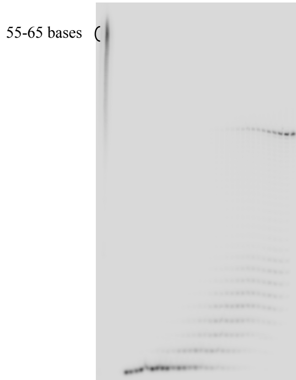
Figure S1: Denaturing PA gel of the RNA substrate, that was purified with the exosome from E. coli cells (left). On the right the bands of an RNase assay are shown that were used for a calibration curve to estimate the size of the RNA on the left.
