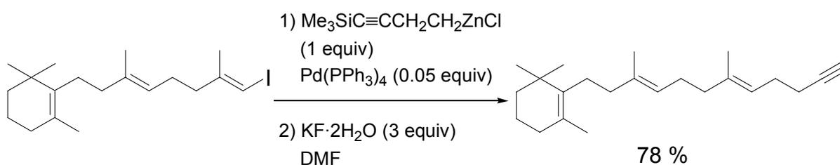
**Scheme 6.** A key step in the synthesis of the triterpenoid mokupalide is the Negishi cross-coupling reaction.
