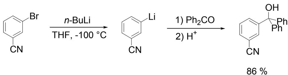
**Scheme 1.** A functionalized organolithium reagent prepared by low-temperature bromine- lithium exchange.
