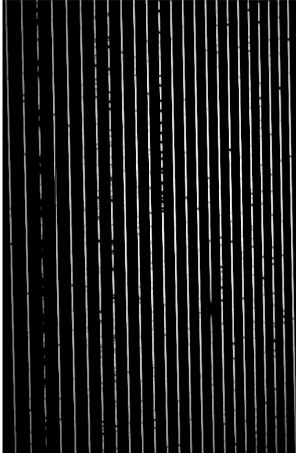
Figure 3.2: Example of a star spectrum observed with the HRS. Each nearly vertical strip corresponds to a spectral order. The wavelength grows from the bottom to the top along a single order and from left to right across the different orders.
