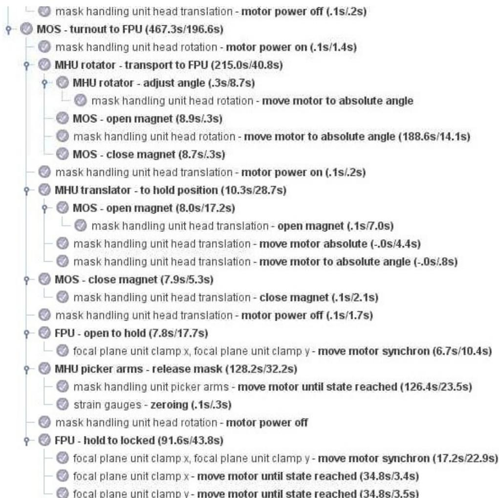
Figure 3.7.: Second part of the Storage-to-FPU Sequence from 'Turnout' to 'FPU'. The beginning of the sequence from 'Storage' to 'Turnout' is shown in figure 3.5
