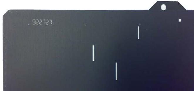
Figure 2.8.: Close up on the mask sheet with mask ID number and mechanical alignment hole on top. The little holes in line below the ID number are for spectral alignment. With the help of these holes one can check the masks orientation with respect to the detector. Three MOS slits are visible on the sheet. The one square hole on the top right is one of several used for alignment of the mask during on-sky acquisition. Field stars are placed in them for alignment.
