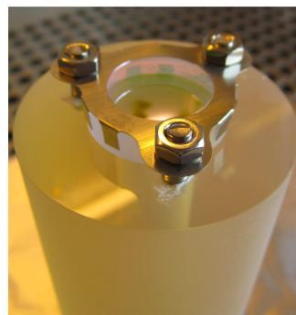
Figure 7.3: Mirror attached to spacer.
