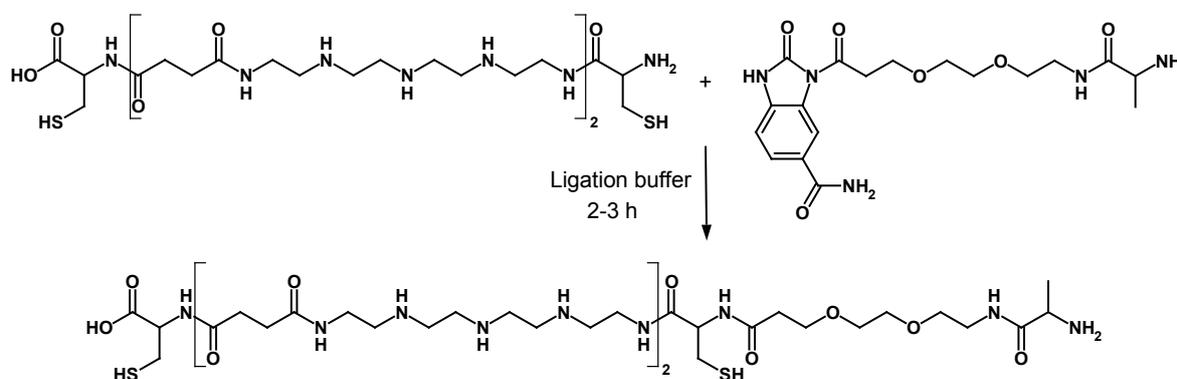
**Scheme 5:** Native chemical ligation of the activated model oligomer A-PEG<sub>2</sub>-Nbz and the polycation C-Stp<sub>2</sub>-C.
