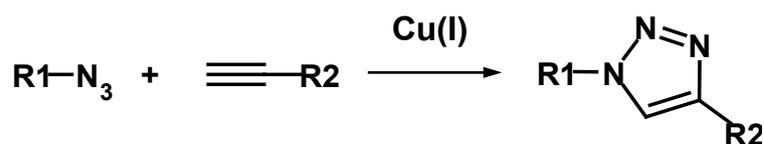
**Scheme 1:** Cu(I)-catalyzed 1,3-dipolar cycloaddition reaction
