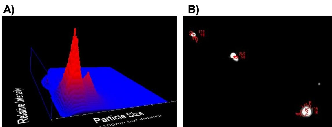
**Figure 29:** NTA of **332** polyplexes in HEPES pH 7.4. A) 3D plot of relative intensity versus particle size. B) Microscope pictures of tracked particles. This experiment was performed by Julia Kasper.
