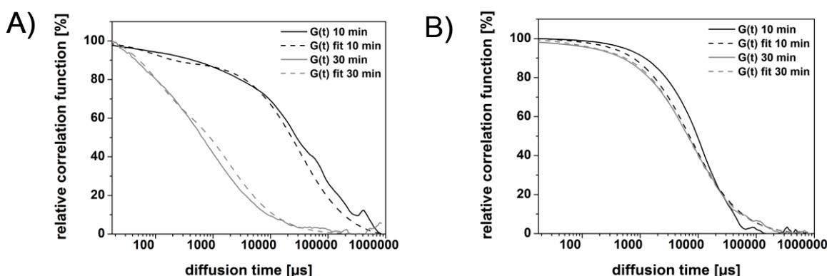
**Figure 31:** Polyplex self-assembly with FCS. Relative correlation functions  $G(t)$  and fitting functions  $G(t)$  fit of A) **49** polyplexes and B) **332** polyplexes after 10 and 30 min.
