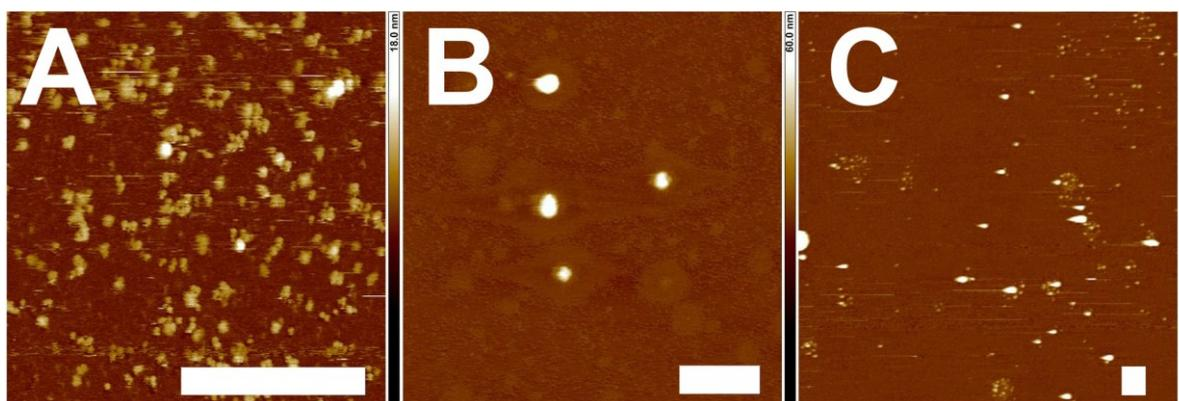
**Figure 28:** AFM pictures of siRNA polyplexes in HEPES pH 7.4. A) **49** polyplexes  $d = 15\text{-}45$  nm; B) **332** polyplexes  $d = 120\text{-}170$  nm; C) **279** polyplexes  $d = 80\text{-}430$  nm. Scale bars represent 500 nm. These measurements were performed by Julia Kasper and Max Scheible.
