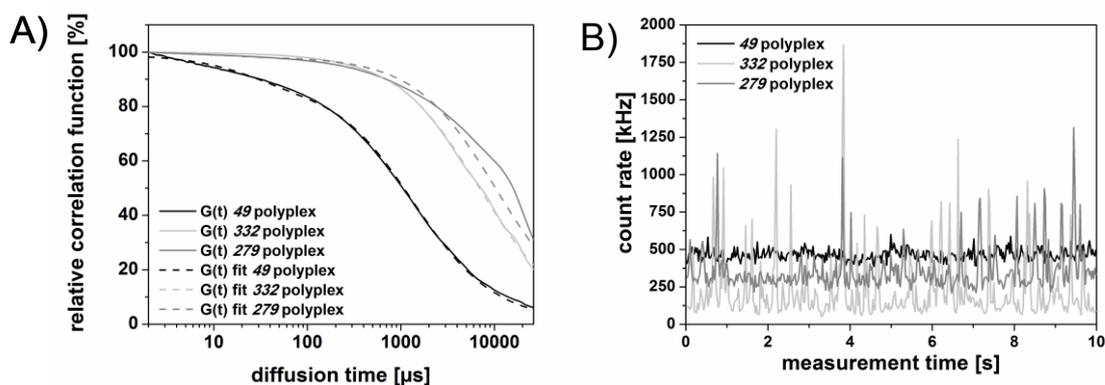
**Figure 30:** FCS measurement of all three polyplexes in HEPES. A) Relative correlation functions  $G(t)$  and fitting functions  $G(t)$  fit. B) Count rate of the polyplexes.
