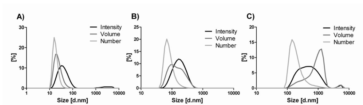
**Figure 26:** Particle size measurement of siRNA polyplexes with DLS in HEPES pH 7.4. Comparison of intensity, number, and volume distribution versus size distributions. A) **49**; B) **332**; C) **279** polyplexes.
