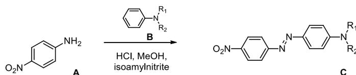
**Standard Procedure 1:** Azo coupling of a *p*-nitroaniline (**A**) with an aniline (**B**) to form the corresponding azobenzene derivatives (**C**).
