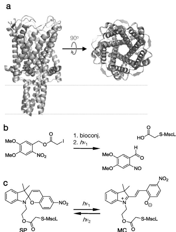
**Figure 20.** Photosensitization of a bacterial mechanosensitive ion channel. a) The structure of MscL in its closed form: side and top view (pdb 2OAR). b) A caged acid used to trigger MscL opening. c) The SP and MC forms of a photoswitch used to reversibly gate MscL.
