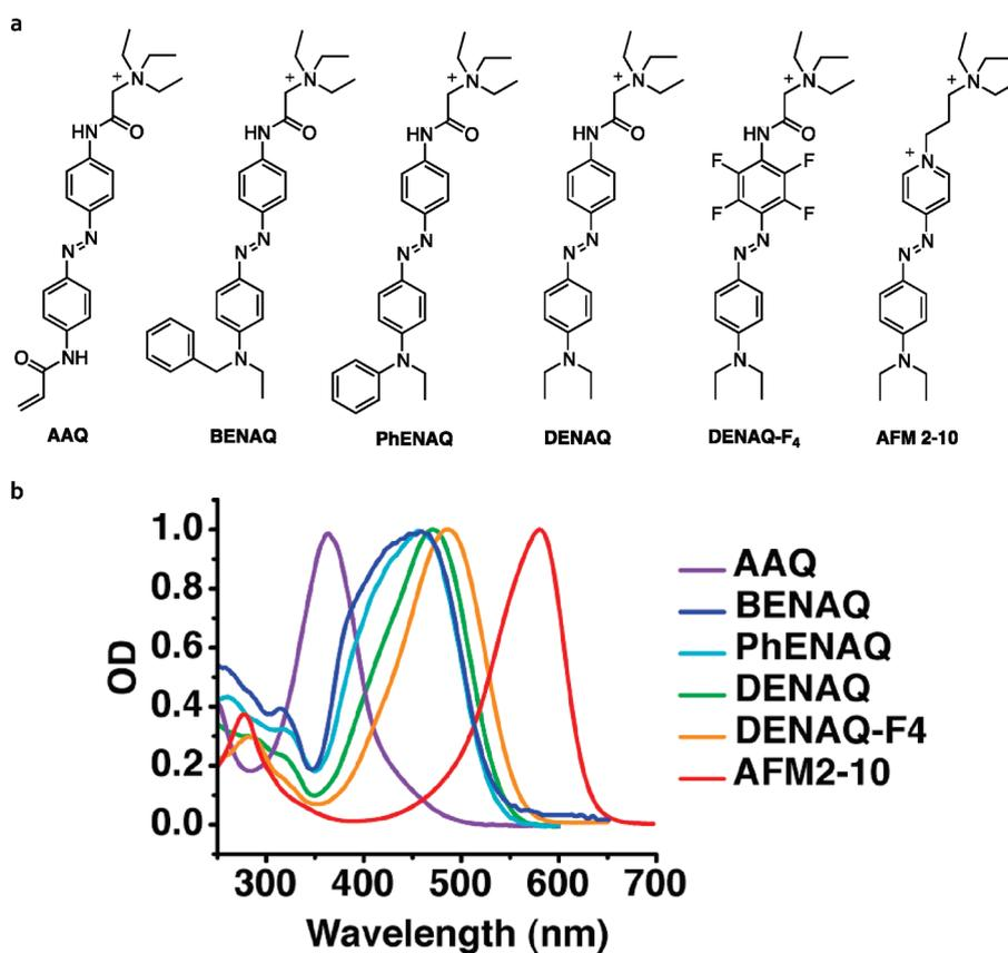
**Figure 2.** (a) Potential photochromic  $K_v$  blockers investigated in this study. (b) UV/Vis spectra of the azobenzenes investigated. Spectra were recorded at room temperature in phosphate buffered saline solution at pH 7.4.
