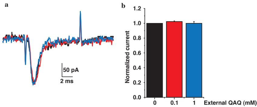
**(a)** Na<sup>+</sup> current recorded from an NG108-15 cell upon depolarization from -70 to -10 mV. Perfusion with QAQ 100 μM (red) or 1 mM (blue) did not alter Na<sup>+</sup> current (black). **(b)** Normalized current ( $0.1 \pm 2.5$  % block  $\pm$  s.e.m.,  $n = 3$  cells,  $p = 0.97$  Student t-test).
