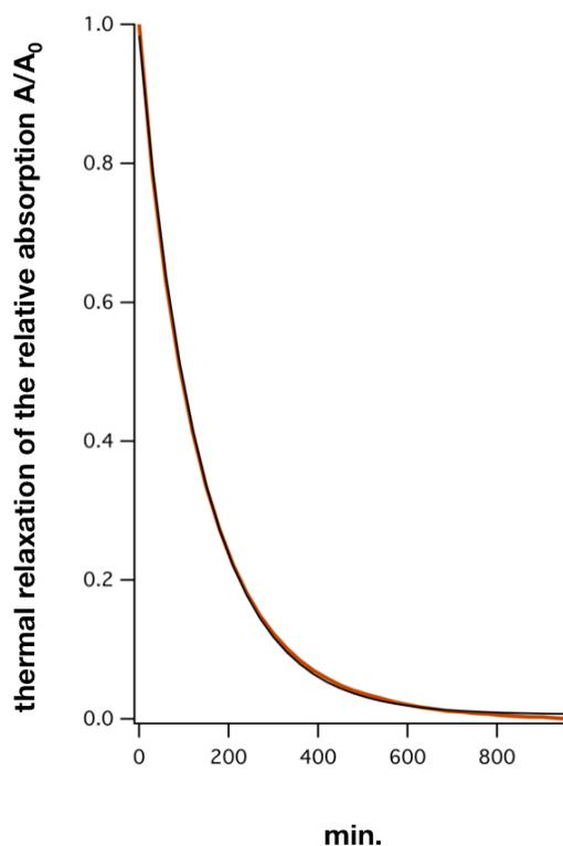
Thermal relaxation of 2,6-dimethoxy-QAQ **1**, measured by an UV-Visible Spectrophotometer in DMSO. Measurement was performed after irradiation with 400 nm. The relative absorption  $A/A_0$  at 403 nm light, is plotted against time. Orange trace represents the recorded absorption. Black trace indicates the course of the fitted exponential function:
