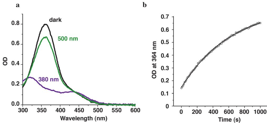
**(a)** UV-Vis spectrum of QAQ in solution (10 mM PBS, pH 7.4) either in the dark, or under illumination with 500 nm or 380 nm light. **(b)** Thermal relaxation of QAQ from *cis* to *trans* in the dark. Data was fitted using a mono-exponential decay ( $t_{1/2} = 449 \pm 5$  s).
