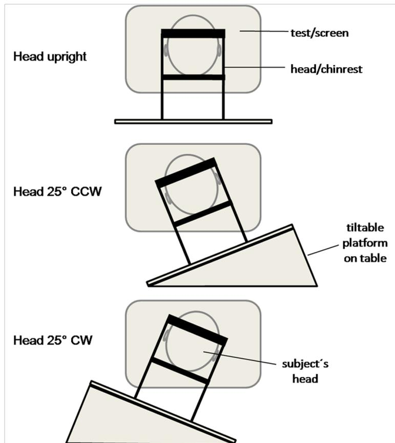
**Figure 2:** Experimental setup in the visual- and tactile-spatial tests in three head orientation conditions: with the subject's head upright ( $0^\circ$  head tilt), or with the head tilted  $25^\circ$  CW or CCW; head position was modulated and stabilized by a tiltable head-and-chin-rest; the head-and-chin-rest was attached to the experimental table (upright head condition) or to a wedge-shaped block on the table (CW or CCW head orientation condition).
