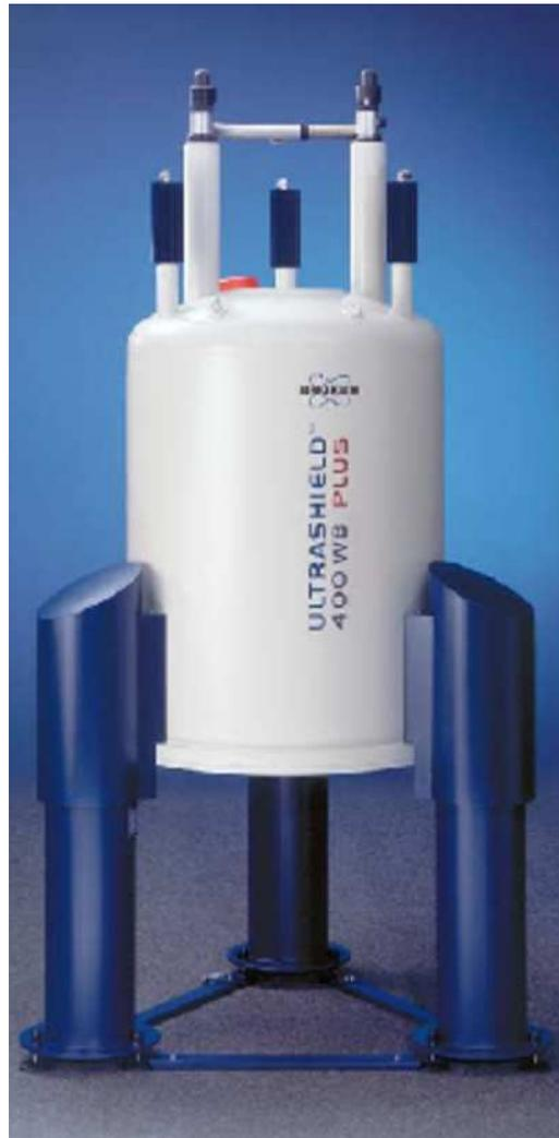
Figure 4.3: A 9.4-T magnet (Bruker Microimaging Systems, Rheinstetten, Germany) was used for the MRI experiment. Its main magnetic field was vertically oriented. The high magnetic field allows microscopy measurements (Picture with kind permission of Thomas Örtner).
